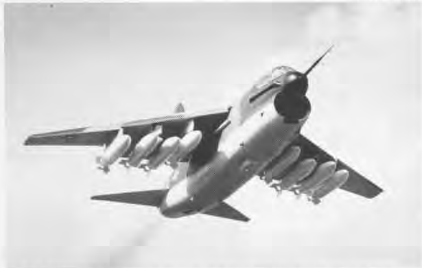
IN THIS PHOTOGRAPH of an A-7D tactical fighter built for the USAF, eight 700-pound ordnance tanks are carried on six wing pylons. The USAF Corsair II is in production at the LTV Aerospace Corporation plant in Dallas. This first released photo of the A-7D was shot from the runway as Chief Experimental Test Pilot Robert Rostine sent the big plane skyward.
