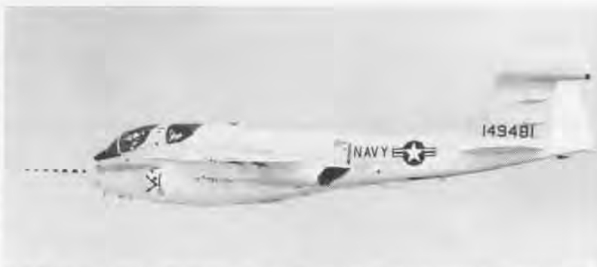
THE NEWEST Intruder, the four-place EA-6B, completed its first flight in May at the Grumman Aircraft Engineering Corporation's Calverton, Long Island, facility. Don King, a company test pilot who flew the aircraft one hour and 45 minutes, declared the flight a complete success. The EA-6B is a twin turbojet, electronic aircraft for carrier and advanced base operations.
