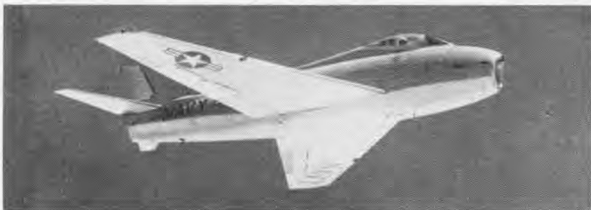
THIS NORTH American-built Navy FJ-4 Fury has shed the traditional seagoing Navy blue for a two-tone gray and white coat. The color scheme, gull gray top and glossy white bottom, extends from air scoop to tail pipe. Powered by a Curtis-Wright J-65-W-4 turbojet, the Fury is capable of speeds in excess of 600 kts. It may serve as a carrier of external weapons.
