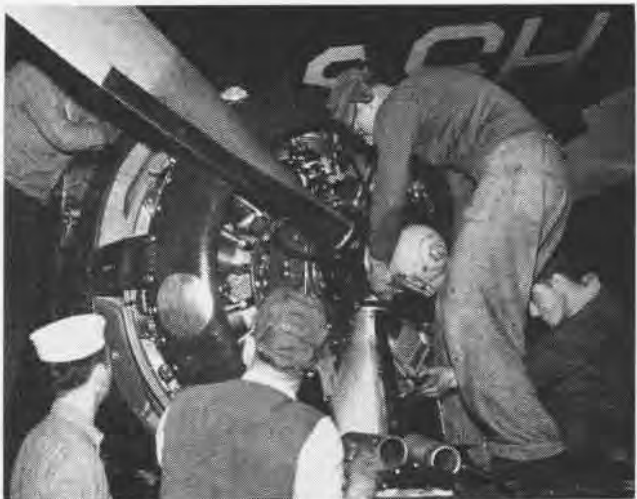
AS THE HUB slides into place, mechs have about finished another engine change. Fast, thorough work kept these planes in 'up' status.
