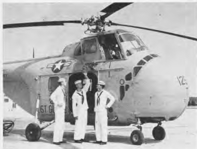
CADETS carefully examine the hoist of a Coast Guard search and rescue helicopter, an HO4S. Pilot sits on right side to operate hoist.
