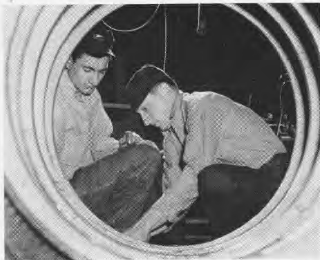
A CHECK against structural failure and repairs to the tail assembly of an F9F-6 Cougar is made by J. Carmichael, AM3, (r) and M. Paster.
