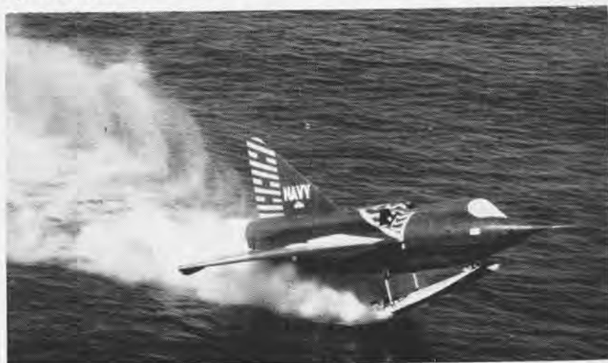
THE EXPERIMENTAL water-based jet fighter, the XF2Y-1 Sea Dart, begins a high speed taxi run on San Diego bay during tests of the single hydro-ski landing gear technique. Other Sea Darts built by Convair have used twin skis. The Sea Dart is powered by twin J-46 turbojet engines.
