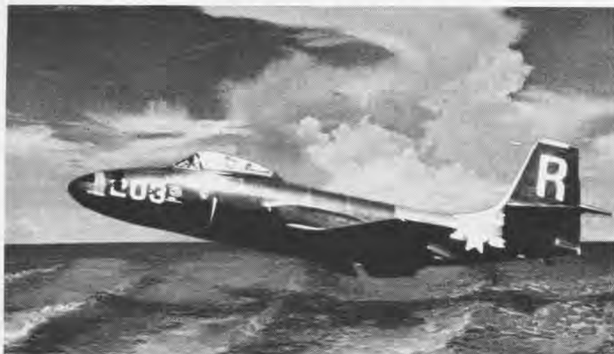
FLAPS DOWN, NOSE HIGH, WHEELS UP, THIS JET IS IN GOOD ATTITUDE TO MAKE WATER LANDING
