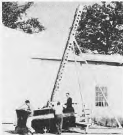
PORTABLE EJECTION SEAT TRAINER 25' HIGH
