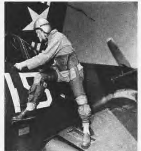
Cutaway type suit covers abdomen, thighs and calves, but gives less G protection.
