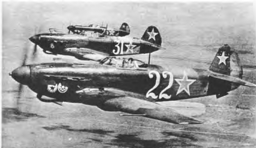
YAK-9 Pointed nose and wings are recognition features of this World War II fighter; wings are wood structure covered with plywood
