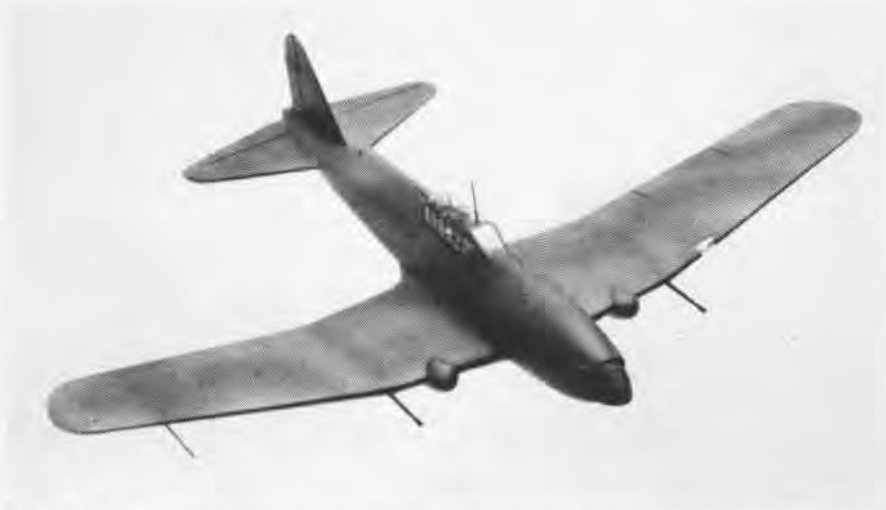
IL-10 Slightly swept-back wings, high canopy feature this armored two-place close support aircraft with 300 mph speed, used against the Germans
