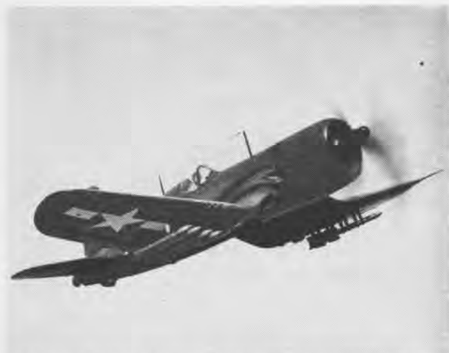
F4U-4 WITH EIGHT 5" ROCKETS ALSO CAN CARRY BOMBS OR TINY TIMS
