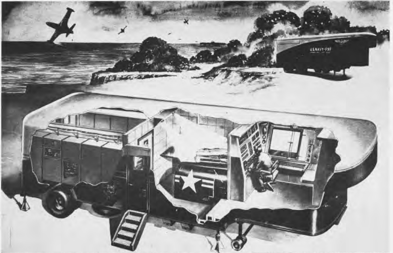
AT LEFT IN TRAINER IS COMPUTER ROOM; IN CENTER THE COCKPIT WITH CLOUD & LIGHTNING PROJECTORS TRAINED ON HOOD; RIGHT, CONTROL ROOM
