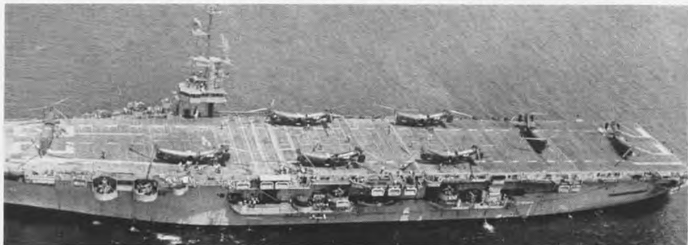
EIGHT PIASECKI FLYING BANANAS SCATTERED ABOUT THE DECK OF CVE PALAU READY TO LOAD TROOPS AND EQUIPMENT FOR BEACH LANDING
