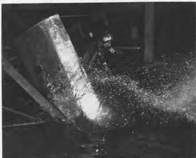
DILBERT Dunker hits water at approximately 30 knots carrying H. E. Blamire, AN. After trainer turns over, he must get out under water.
