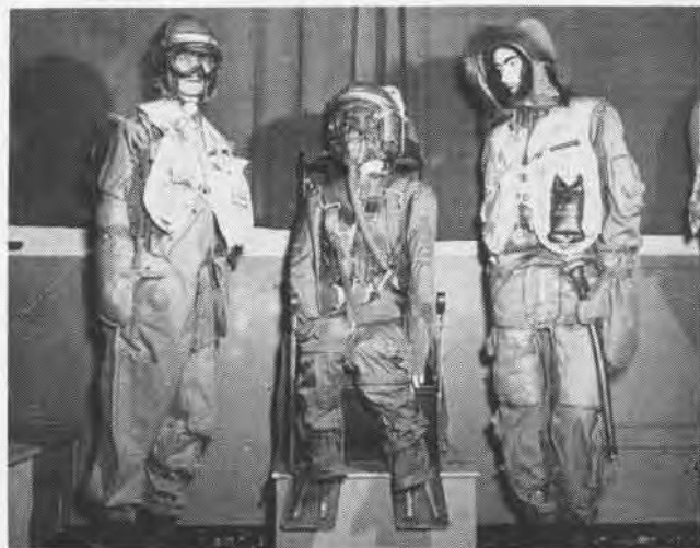
ANTI-G suit seated in an F9F ejection seat is flanked by the M-3 and M-4 exposure suits. FAETULant covers all phases of survival.
