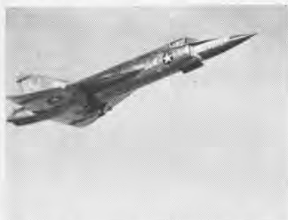
POWERED by a P&W J-57 engine with afterburners, Convair's modified version of the Av Force F-102 delta-wing all-weather interceptor, was flown supersonically six months after design and manufacture. It's designated F-102A.
