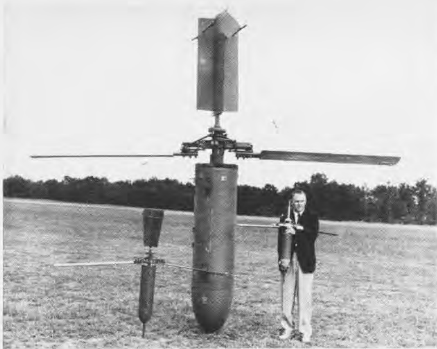
ROTOCHUTE IS NEW ADOPTION OF MARINE CORPS FOR PINPOINTING AIR SUPPLY DROPS
