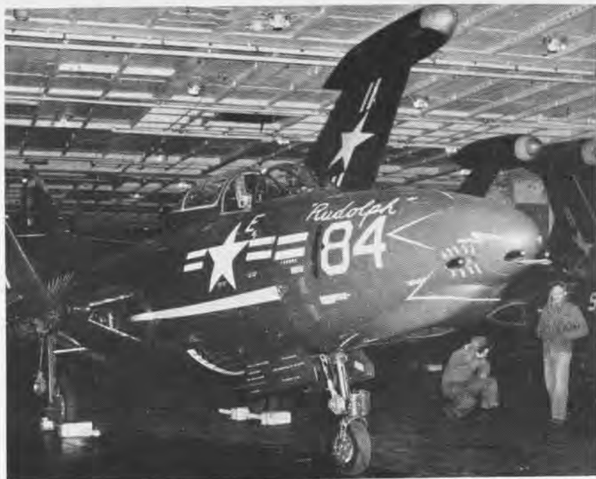
THIS strange looking beast is a Panther/Cougar and belongs to VF-84 aboard the USS Champlain . Sporting a Panther fuselage and a red-tipped Cougar nose shell, the plane was a conundrum until it was discovered that VF-61 had replaced a damaged nose section with a nose shell from one of their planes during the night. LCdr. H. V. Ladley is CO of VF-84, Cdr. J. Thomas, VF-61.
