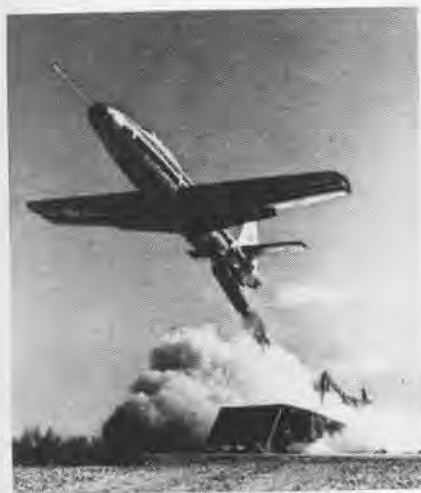
ASSISTED by a booster rocket, similar to that used by the Matador, a piloted AF jet fighter is launched at flying speed from a zero-length launcher developed by Martin Co.
