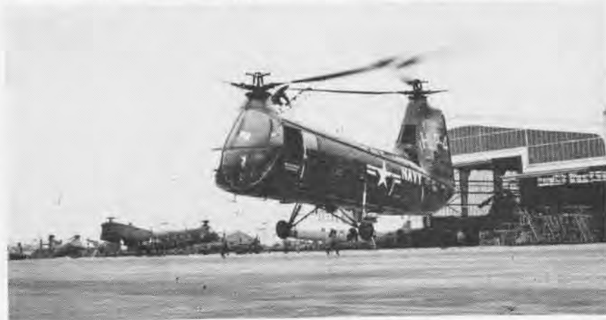
RE-DESIGNATED HUP-4 , this production model Piasecki HUP-2 with a new engine installed has passed its first flight successfully at Philadelphia International Airport. Powered by a Wright R-1300-3 engine, the HUP-4 will have higher payloads, speeds, and ranges than its predecessor.
