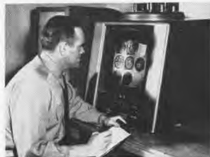
STUDENT test pilot takes instrument data from flight-exposed panel film at Patuxent.
