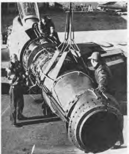
AFTERBURNERS , like this on a P&W J-48 turbojet engine, create new jet noise problem.
