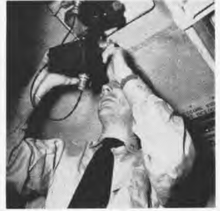
STAR SIGHT for night navigational fix is taken during the Azores-Paris leg of flight.
