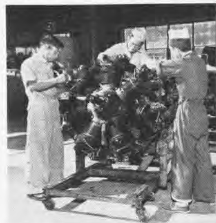
RADIAL engines such as this R-670 also must be repaired at Formosan air station.
