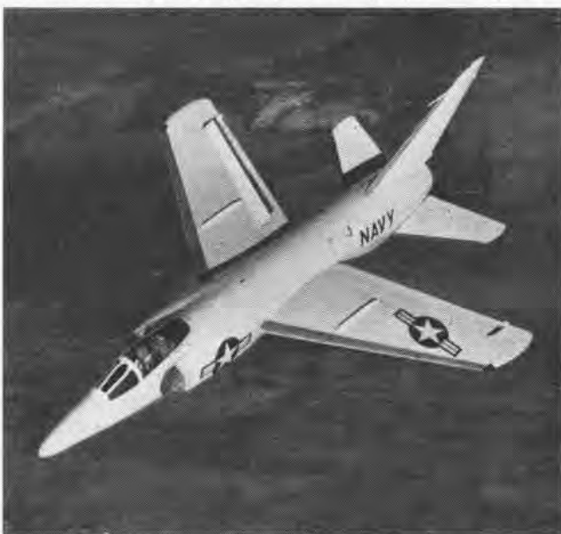
COKE BOTTLE DESIGN WAS INCORPORATED IN THE F11F-1 TIGER
