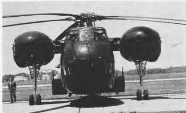
POWERFUL TWIN-ENGINE HR2S HAS RETRACTABLE LANDING GEAR
