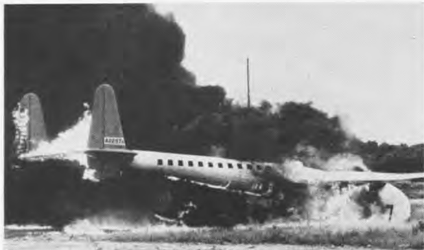
A SERVICE-WEARY C-82, WITHOUT INERTING SYSTEM, FIRES AFTER CRASH LANDING
