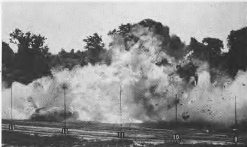
CRASH FIRE RESULTS IMMEDIATELY IN AN F-84 FIGHTER WITHOUT INERTING SYSTEM
