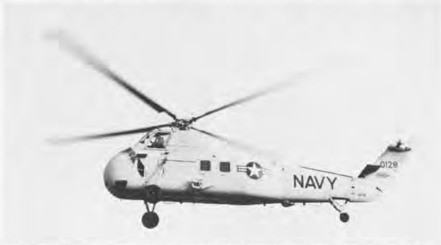
SIKORSKY S-58 WILL SERVE AS A FLIGHT TEST VEHICLE FOR T-58 TURBOSHAFT ENGINE
