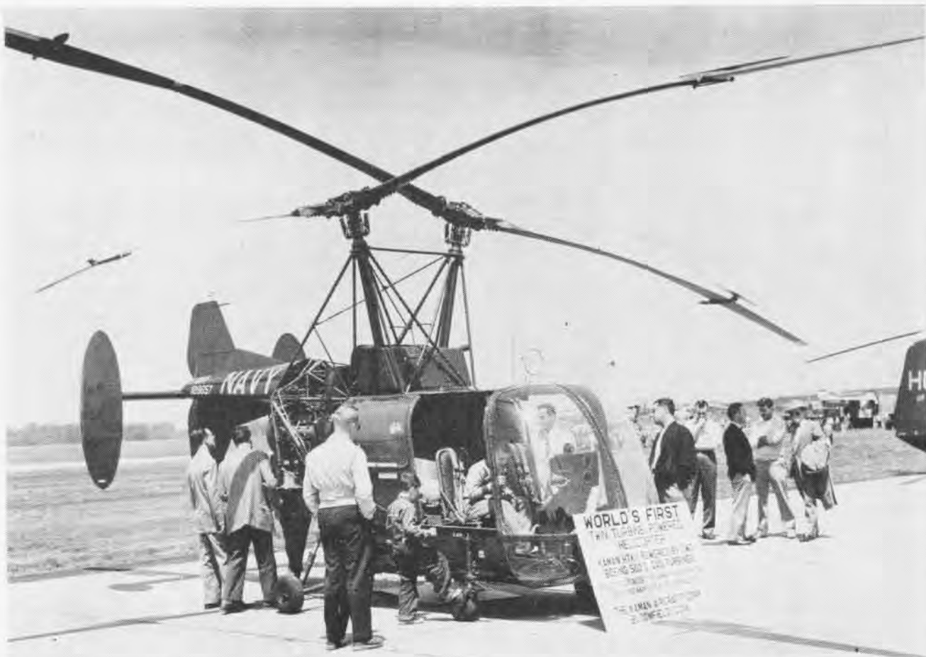
KAMAN'S HTK-1, RESCUE AND RECONNAISSANCE CRAFT, HAS FIRST TWIN GAS TURBINES AND FIRST TWIN INTERMESHING ROTORS.
