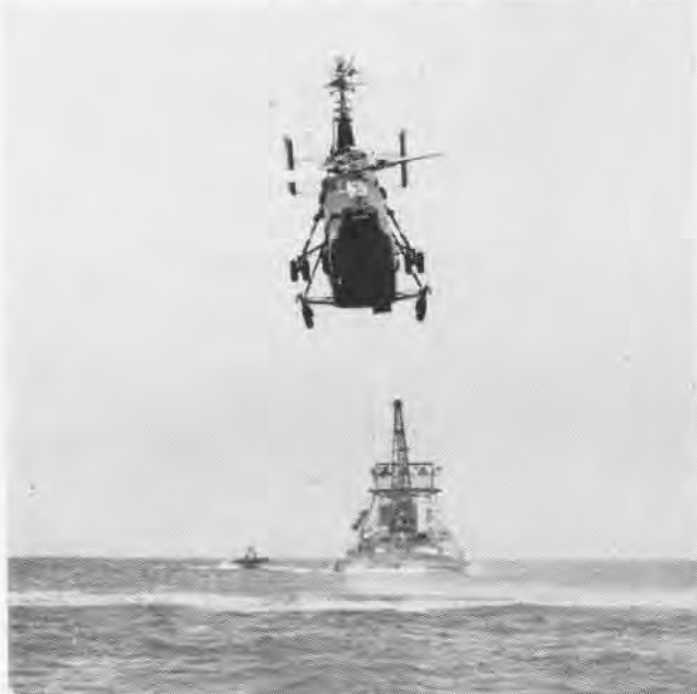
HSL-1 SHOWS TOWING STRENGTH AS IT PULLS 300-TON DERRICK
