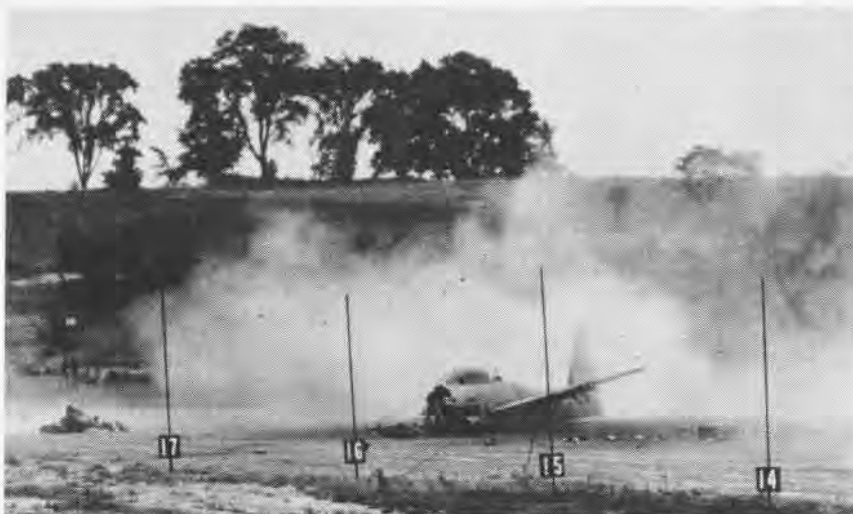
IN CRASH OF SAME TYPE FIGHTER WITH THE INERTING SYSTEM, NO FIRE RESULTED
