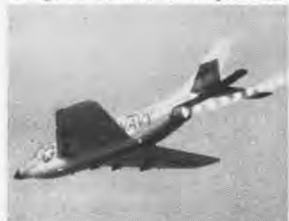
THIS IS an unusual photograph showing "sbock heads" in the exhaust trail of the Demon's J-71-A-2 turbojet engine. Common in rocket engines, it is a phenomenon in turbojets.
