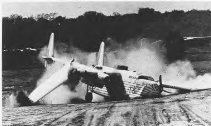
AFTER GROUND LOOP CRASH OF THIS C-82, INERTING SYSTEM STEMS FIRE OUTBREAK
