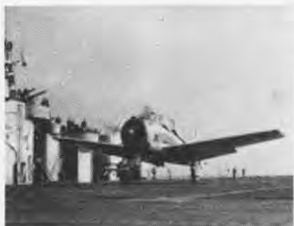
THE NAVY'S new trainer, the T-28C, picks up a deck pendant during carrier qualifications aboard the USS Forrestal. Seconds later, as observers stood by, the T-28C's pilot added power, and the two-place trainer commenced a take-off from the big carrier's angled deck.
