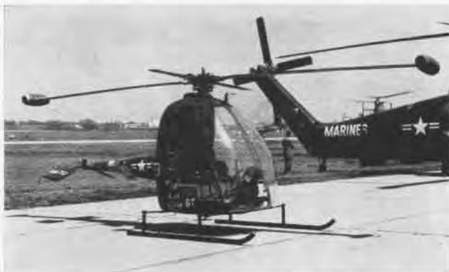
SMALL 12-POUND RAMJET ENGINES DRIVE THE HILLER HORNET
