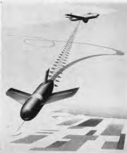
GRAPHIC illustration of how the system works shows ground pilot airplane in control during flight. In landing, pilot station in control during missile's take off. Drawing shows airplane brings missile in part way, ground station takes over.
