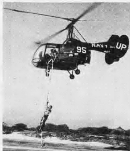
A 20-FOOT RESCUE LADDER MADE OF NYLON
