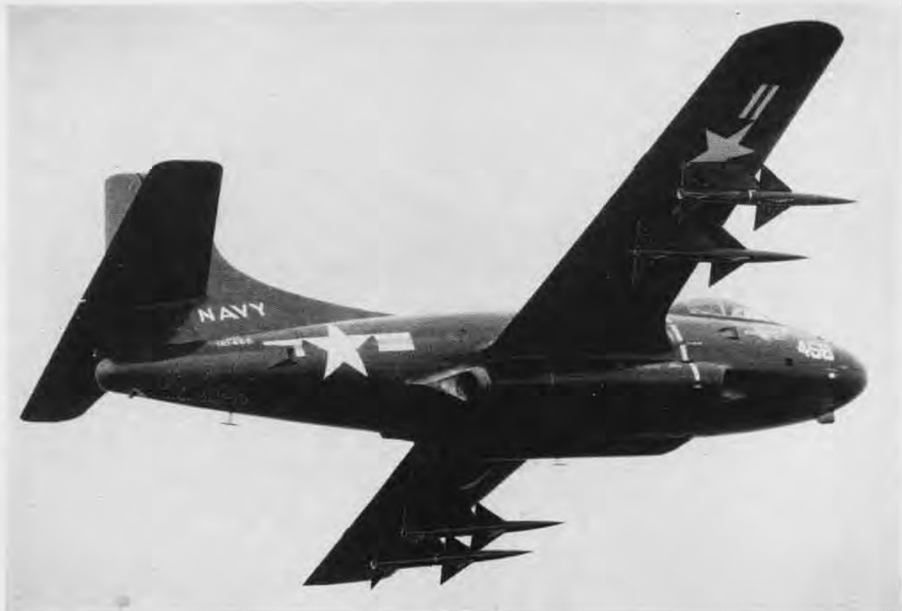
FOUR SPERRY SPARROW AIR-TO-AIR GUIDED MISSILES HANG FROM RACKS ON NAVY'S TWIN-JET NIGHT FIGHTER, DOUGLAS SKYKNIGHT
