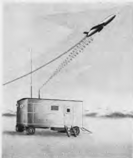
GRAPHIC illustration of how the system works shows ground pilot airplane in control during flight. In landing, pilot station in control during missile's take off. Drawing shows airplane brings missile in part way, ground station takes over.
