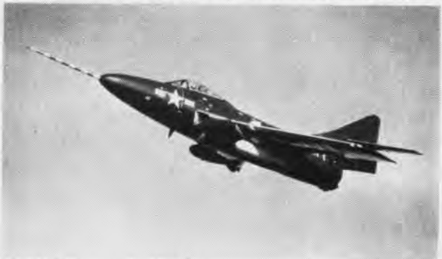
GRUMMAN'S versatile F9F-6 Cougar jet is shown in first photo released with two externally-mounted 1,000-pound bombs added.
