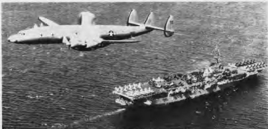
THE NAVY'S sky-an-sea-fighting team, a Lockheed WV-2 flying-eye radar plane and the carrier load of planes it can direct into battle when it spots danger in front of the fleet. The big plane has a wing spread of 123 feet and carries 31 men. Day or night, the WV-2 crew can keep watch on the outskirts of a task force.
