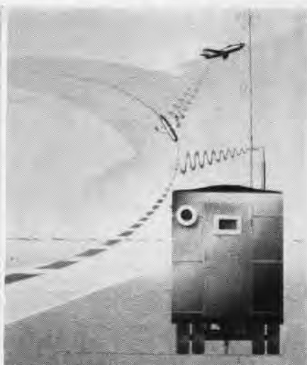
GRAPHIC illustration of how the system works shows ground pilot airplane in control during flight. In landing, pilot station in control during missile's take off. Drawing shows airplane brings missile in part way, ground station takes over.
