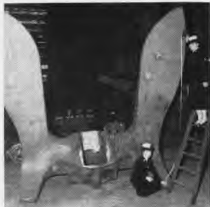
BLADES of the largest anchor ever built by the Navy measure about 12 feet as demonstrated by Frances Gand, SKSN, and Iris Mae Bixby, SA, at Norfolk Naval Shipyard Foundry. Two of the 60,000-pound giants are slated for Navy's latest carriers USS Forrestal and USS Saratoga.
