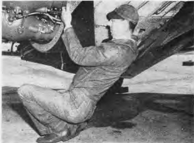
A MAN with "feel", O. S. Kelly, ADC, adjusts high pressure fuel pumps with arm in accessory section for a minute adjustment.
