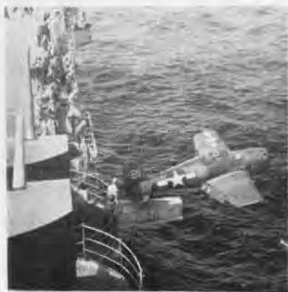
UNUSUAL event of WWII is F6F being catapulted from the hangar deck of the Hornet.
