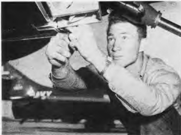
SOMETHING almost new to the line of maintenance crew is a hydraulic leak which J. R. Hornsby, AMAN, concentrates on repairing.
