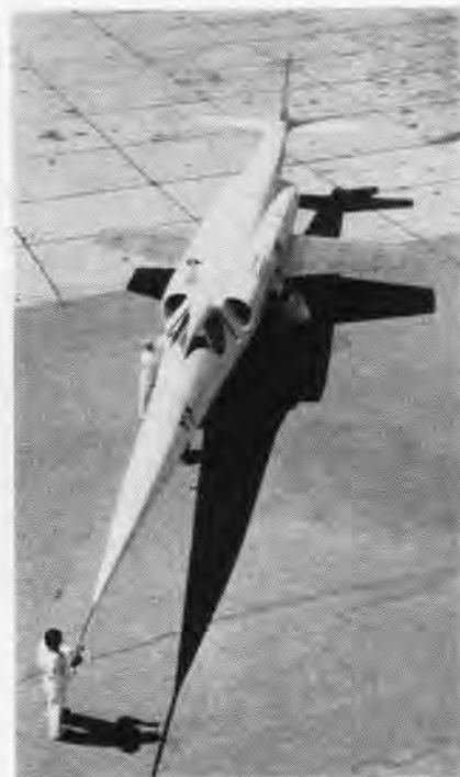
LATEST of the nation's research aircraft to be unveiled is the Douglas X-3 "Stiletto," sponsored jointly by Navy, Air Force and NACA for extreme high speeds and altitudes. Slightly heavier than an R4D, its wing-span is less than that of an R4D's tail—22'. It is 66 feet long. Carries 1200 pounds of instruments. Two jets power it.
