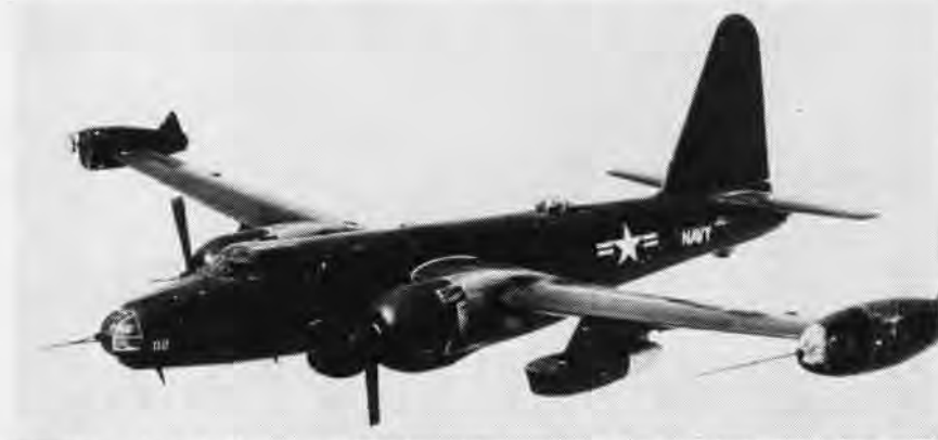
THE P2V , which holds the world's long-distance flying record of 11,238 miles, now enters the speed ranks by adding two jet engines in pods under its wings, a la Boeing bombers. Two Westinghouse J-34 jets are shown carrying the load while the props on Neptune's regular turbo-compound engines are feathered. The jets will up the P2V's speed.
