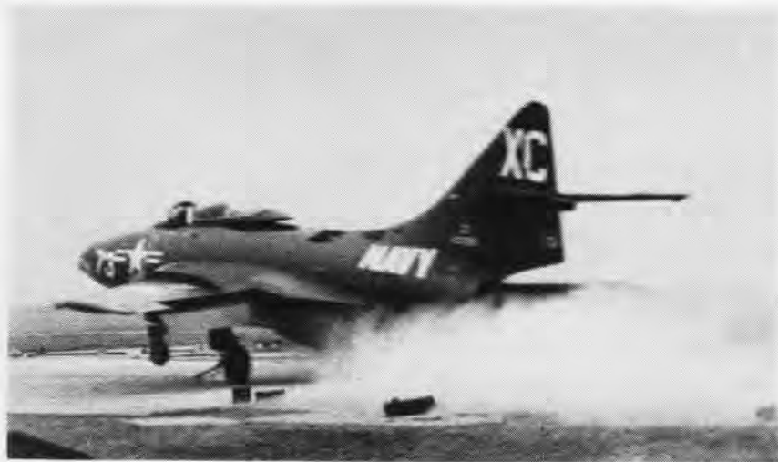
FIRST launch of the new steam catapult at commissioning ceremonies is made by a Navy F9F-6 Cougar. Steam drifts from the catapult track as plane begins to move.
