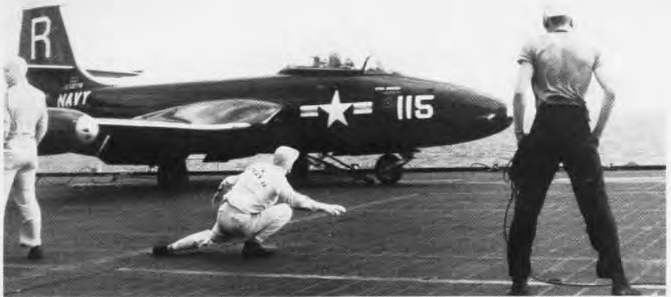
WITH THE advent of jet aircraft aboard carriers, catapult takeoffs became the normal procedure. Catapult officer gives signal to launch Banshee on Coral Sea. Heavier and faster planes are making this type of catapult an obsolete piece of machinery.
