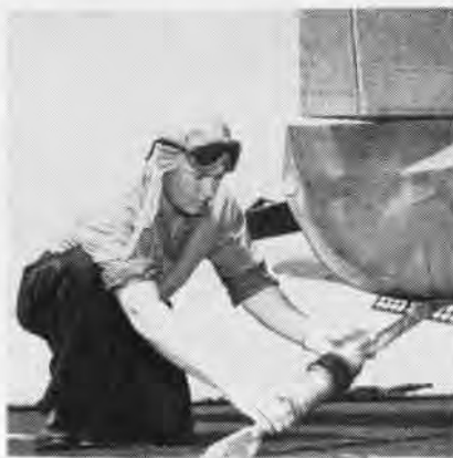
FLIGHT deck crewman adjusts the retaining ring prior to launching from Independence .
