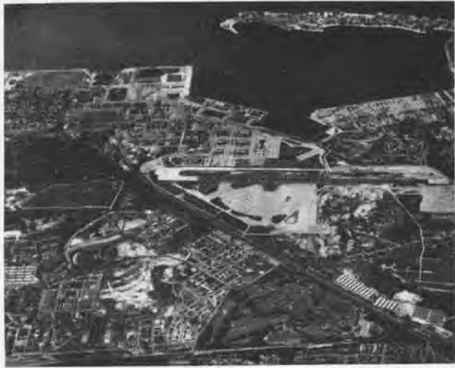
HERE IS the station as it looks today, covering 2150 acres. Forty per cent of the land comprising the base was reclaimed, drained and filled.
