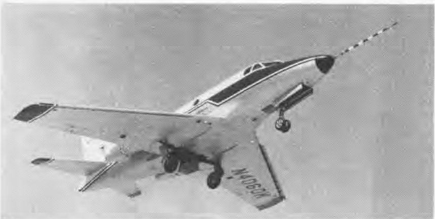
A NEW RECOGNITION item in U. S. skies is North American Aviation's Sabreliner which made its first flight recently. The twin-jet utility trainer can carry 10 passengers; weighs only 15,330 pounds. Powered by GE J-85 turbojets, the pressurized Sabreliner has a cruising speed of 500 mph at 45,000 feet; can make it from Los Angeles to New York with one refueling. Developed for specific requirements, aircraft was designed for AF pilots to maintain flying proficiency.
