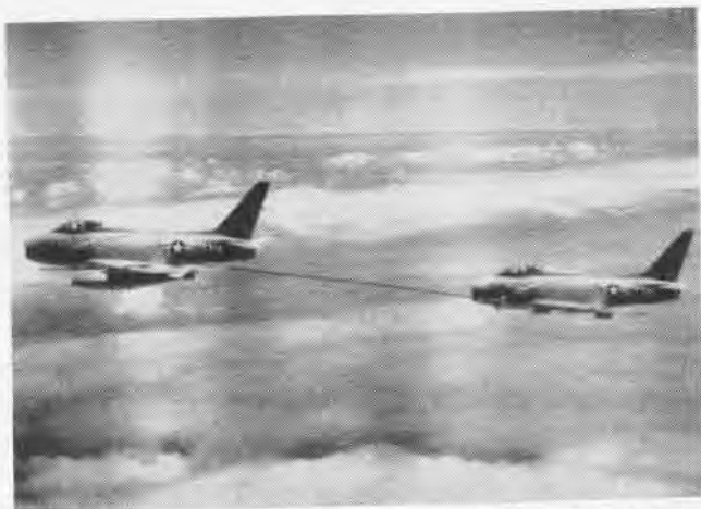
Buddy Tanker Refueling System on operational flights. Use of probe-drogue engagement method enables consistent hook-ups even under conditions of turbulence, low visibility, altitude and darkness.
