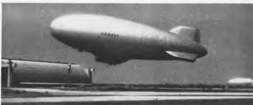
WASH-AND-FAST-DRY materials are all in fashion. Dacron goes over big as it proves popular with lighter-than-air designers. Here a Navy airship using a dacron fiber envelope takes off from NAS Lakehurst, New Jersey. The ZS2G-1 is the newest type airship to use dacron envelope.
