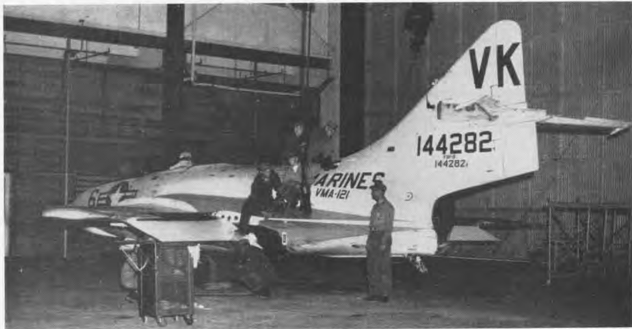
MARS-37 ASSEMBLY SHOP MEN READY A COUGAR FOR OVERHAUL. THE F9F-8 WILL LEAVE THE SQUADRON IN PRIME CONDITION.
