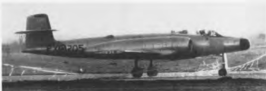
CANADIAN CF-100 interceptor, speeding down runway at more than 100 mph, is shown a few seconds after its nose wheel engaged the emergency overrun safety arrester during a test at Uplands Airbase near Ottawa. The actuating cable has snapped into action a lower steel cable which is about to catch the main landing gear. The arrester has stopped the 34,000-pound jet at aircraft speeds up to 150 knots. It will be installed at seven Canadian airports.
