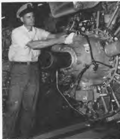
GABBARD TRIES FIX ON R-3350-34 ENGINE
