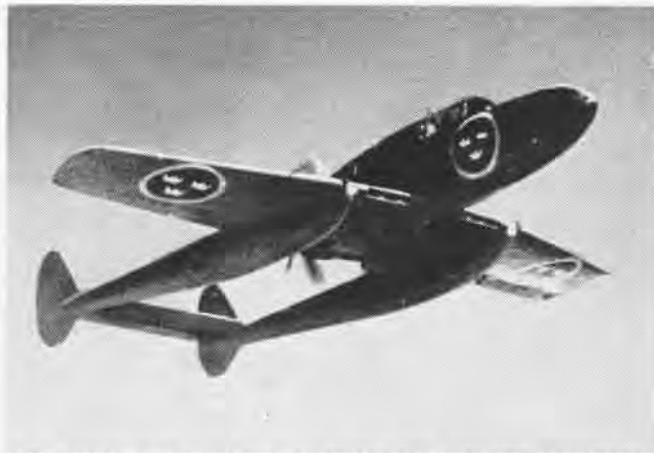
J 21 BEETLE, A PUSHER TYPE FIGHTER, HAS TURBOJET COUNTERPART
