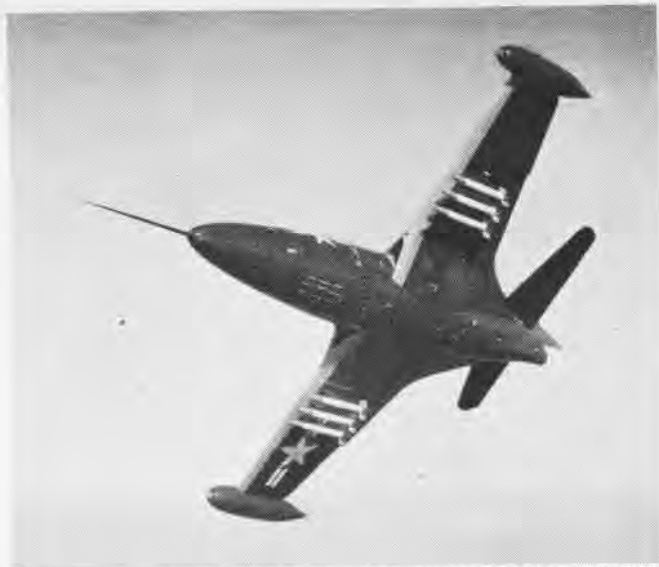
F9F'S SPEED BRAKES ARE PERFORATED AREA ON BELLY AHEAD OF WING
