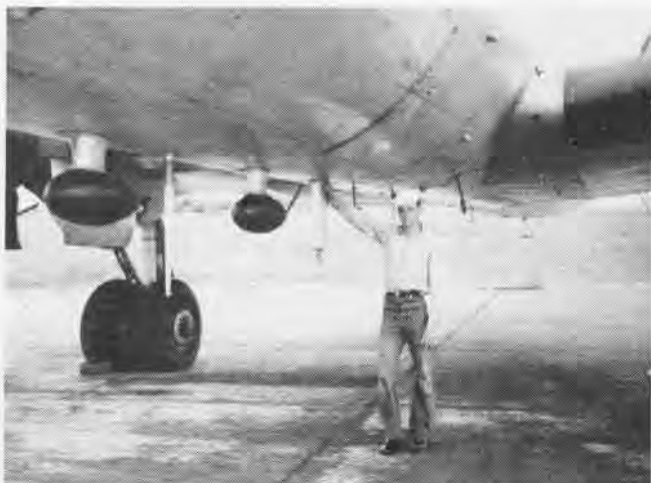
UNDERSIDE OF PLANE IS LINED WITH ANTENNAS; SOME ARE ON TOP TOO
