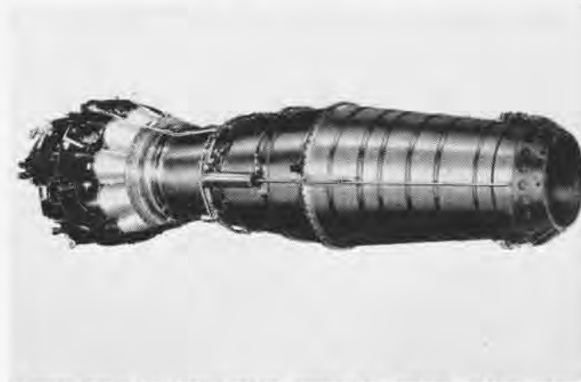
J-48 IS MOST POWERFUL PLANE TURBO-JET ENGINE FLYING TODAY
