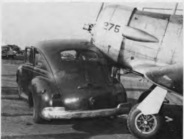
ARMY car stopped in taxiway to ask directions. At the same time pilot of SNJ failed to zig-zag to the clear area just a few feet away.
