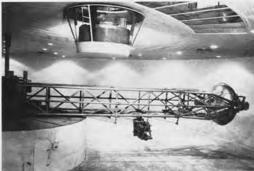
OPERATOR IN BLISTER NEAR CEILING IS READY TO OPERATE THE CENTRIFUGE PLATFORM
