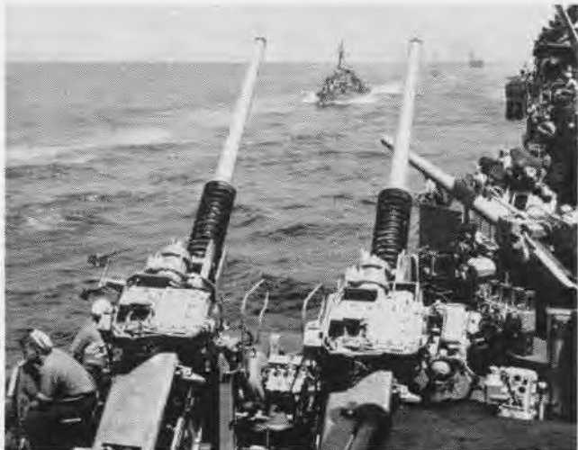
ANTI-AIRCRAFT defense for carriers is supplemented by the vessel's wicked twin 3-inch 50 cal. and 5-inch 38 dual-purpose deck weapons.
