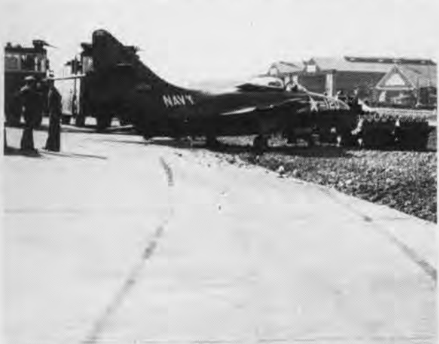
EXCESSIVE taxi speed caused Panther to swerve off runway after travelling 180 feet braking and smashed the left wing on tractor.
