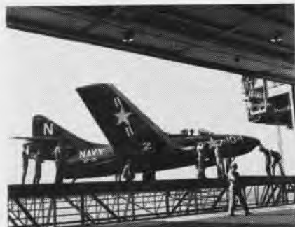
DECK EDGE elevators move fighter planes efficiently during all re-spotting operations.
