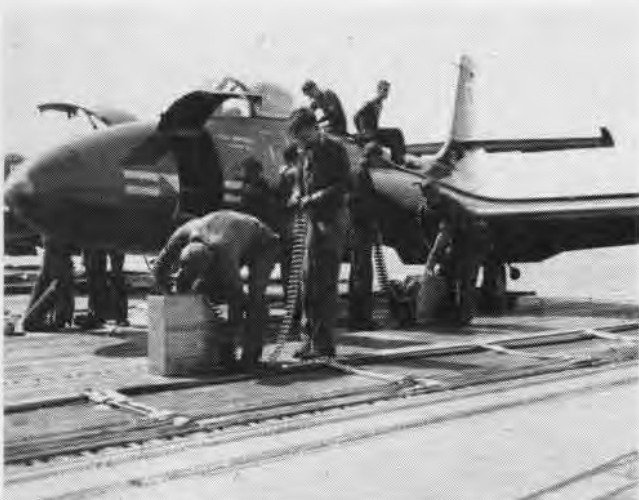
ORDNANCE personnel load 20-mm magazines for a Banshee jet. Four gun ports in the nose constitute the destructive firepower of this F2H.
