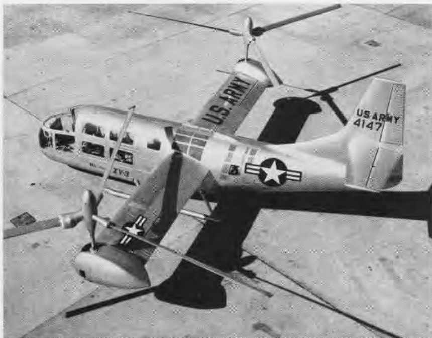
DESIGNED FOR HIGH CRUISING SPEEDS, THE XV-3 SPORTS THE TILTING ROTOR DESIGN
