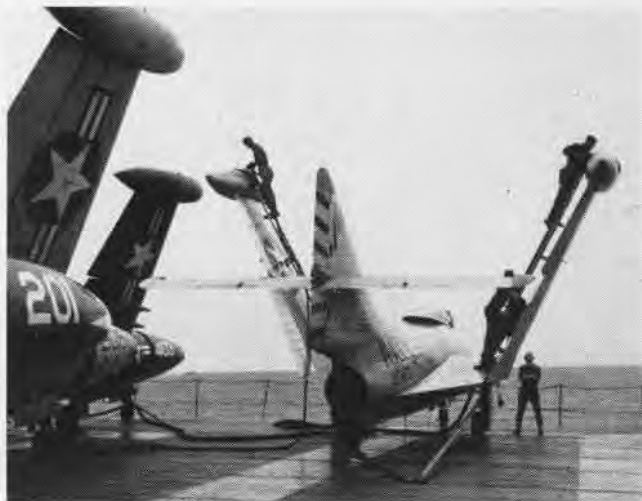
FUELING of a Grumman Panther jet is a step in assuring the accomplishment of the fighter aircraft's mission. Wing tanks extend plane's range.
