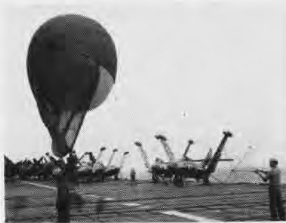
PRIOR to take-off of carrier aircraft, two aerographers release balloon for wind test.
