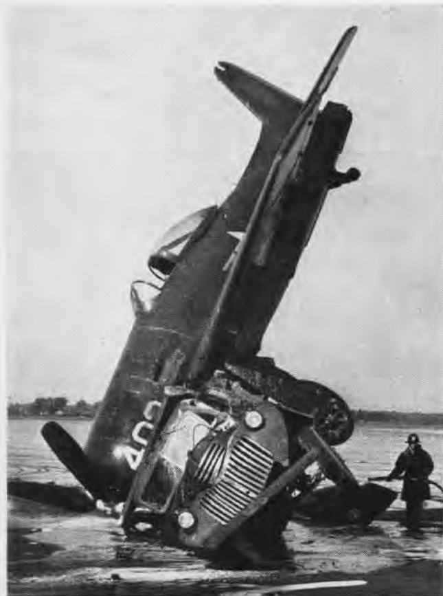
BEARCAT came a cropper as a result of poor brakes which caused it to slew off and run into a truck parked too close to runway.
