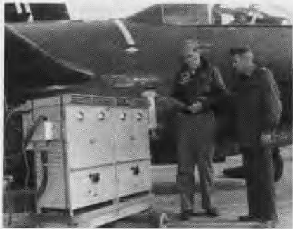
LCOL. T. J. O'Connor, CO of VMF(N)-513, inspects a portable rectifier used as a power source for checking electronics gear in F3D-2 aircraft. The system was ingeniously designed by CWO E. A. Marx (r).
