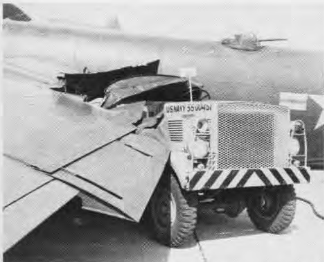
MY ACHING back! NC5 mobile starter protrudes from wingroot of Neptune which settled from landing gear malfunction at starting.
