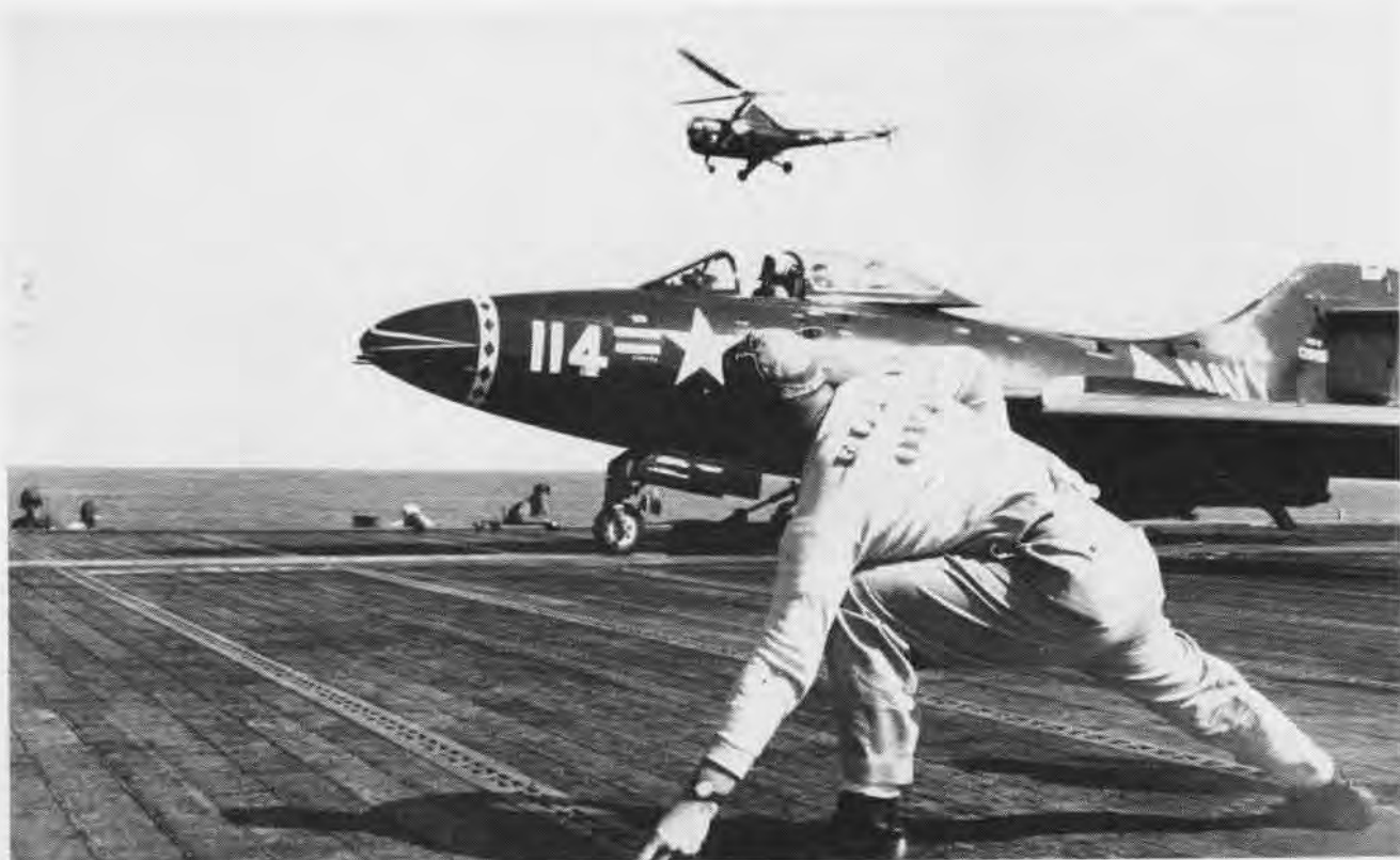
AN F9F-6 Cougar pilot is given the 'launch' signal by the carrier's catapult officer as a Sikorsky helicopter hovers in the background on plane
