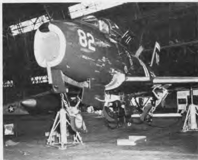
IMPORTANT part of maintenance is drop test of landing gear. Here, crewman watches indicator as landing gear goes up on new FJ-3 Fury.
