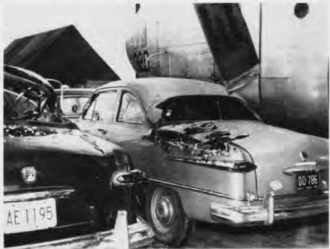
OVER-CROWDED parking lot occurred when this R40 jumped the chocks during engine turn-up and battered five unoffending cars nearby.
