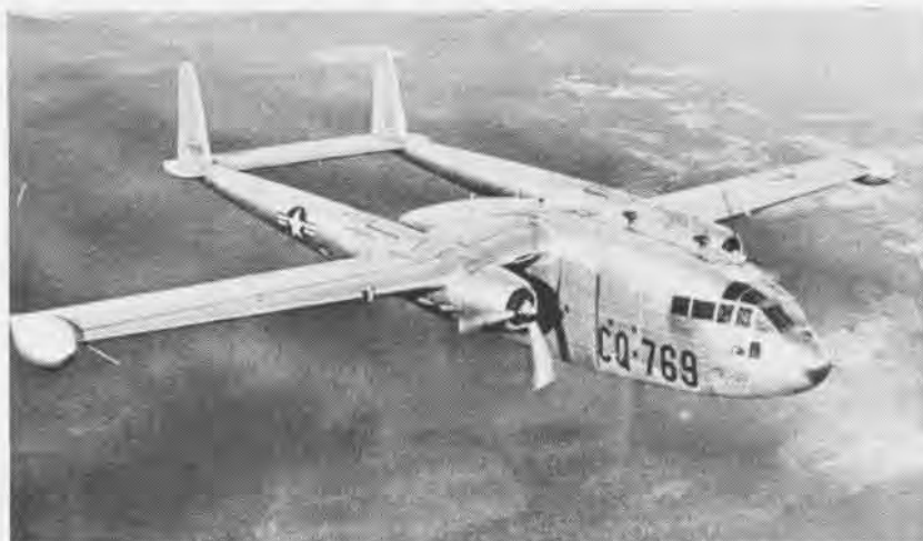
MARINES WILL FLY THE FAIRCHILD R4Q PACKET WHEN IT REACHES THE FLEET; BIG FUSELAGE, TWIN BOOMS HELP RECOGNITION
