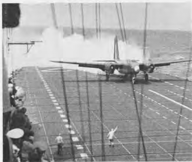
Opening up its JATO bottles, a P2V Neptune powders deck with white as it thunders down for takeoff to fly nonstop to Moffett Field, Cal.
