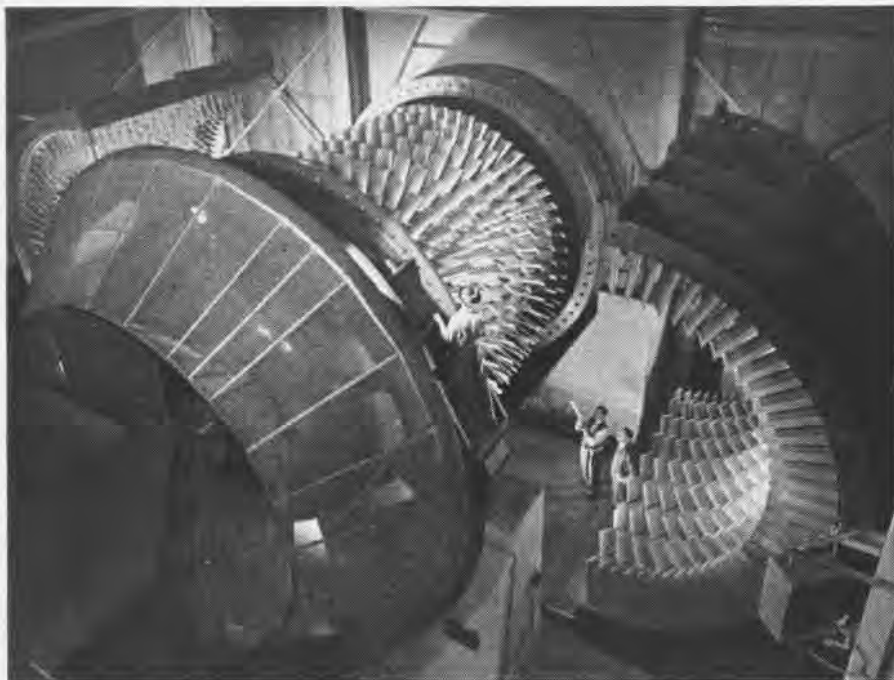
Are those pygmies working around the axial compressor blades of a jet engine? No, the men are inspecting the giant rotor blades of NACA's new 8x6 foot supersonic wind tunnel
