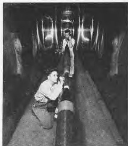
Scientists at Cleveland install a model in the new supersonic wind tunnel for testing
