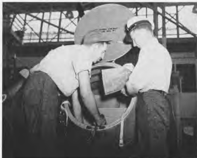
NOSE TANKS ARE INSTALLED IN SNB-55 FOR LONG WEATHER FLIGHTS
