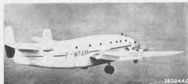
BREGUET 761 TWIN RUDDERS AND THIN AFTER FUSELAGE DISTINCTIVE
