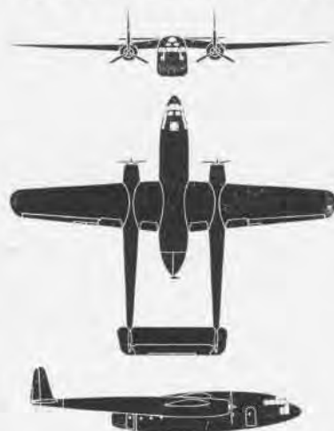
MARINES WILL FLY THE FAIRCHILD R4Q PACKET WHEN IT REACHES THE FLEET; BIG FUSELAGE, TWIN BOOMS HELP RECOGNITION
