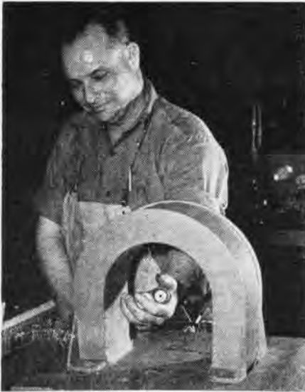
Demagnetization is necessary first to allow the removal of steel particles
