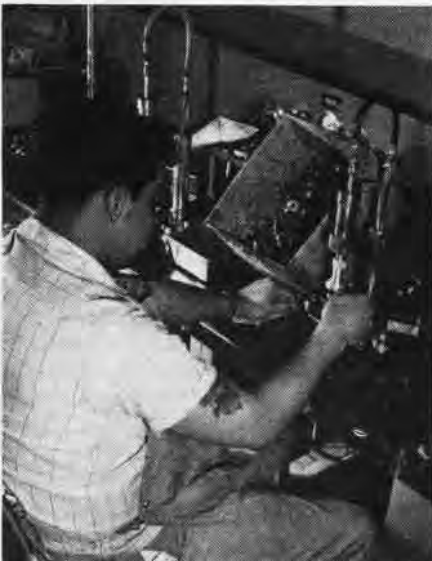
Pressure relubricators force fresh grease into and through clean bearings
