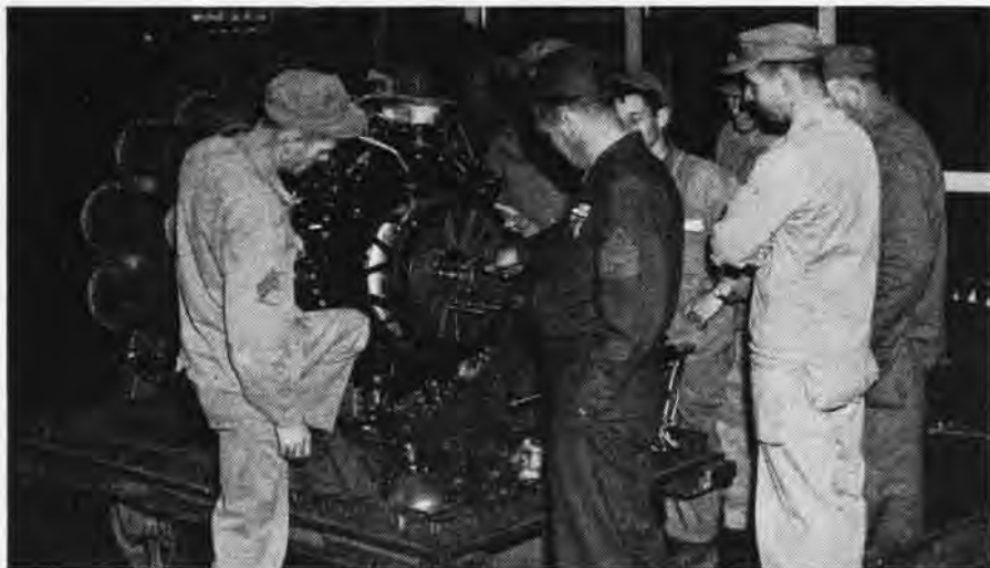
ENGINEERING COURSE STUDENTS LEARN OPERATION OF I-16 JET ENGINE WHICH DROVE RYAN FR-1
