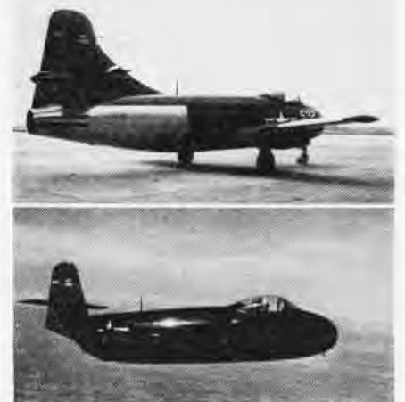
F6U AT TOP HAS TAILPIPE AFTERBURNER ADDED
