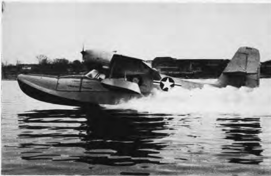
NOT A NEW TYPE AMPHIBIAN BUT JUST A MODIFIED WIDGEON WITH THE PSM HULL INSTALLED
