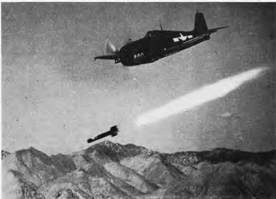
Squirting a tail of flame 50 feet long, a 11.75" aircraft rocket, the Tiny Tim, takes leave of its moorings on the belly of an F8F over the barren California hills near Naval Ordnance Test Station at Inyokern. The Tim is the largest aircraft rocket in use today, with a 4000-yard slant maximum range. Weight 1173 lbs., length 114".
