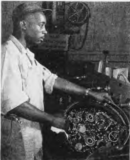
Bearings are mechanically agitated in baskets immersed in solvent bath
