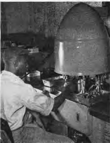
In rapid spinning warm oil flushing machine, bearings get final cleaning
