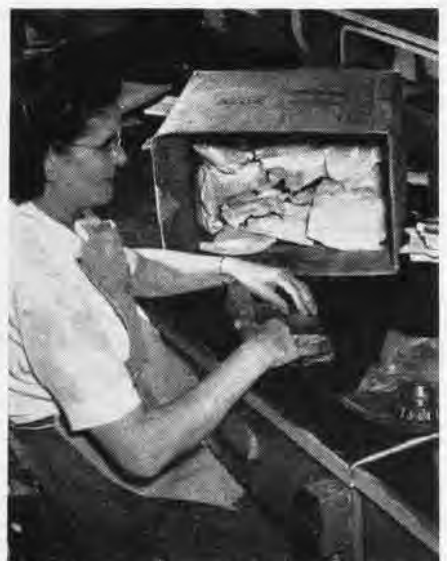
Finally each bearing is wrapped and sealed in pre-labeled foil barrier bag
