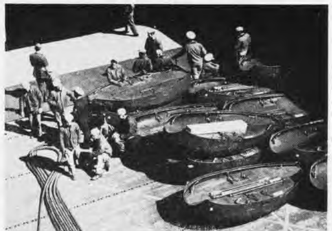
Auxiliary belly gasoline tanks for FH-1 are of special design; here a cluster of them are carried up the forward elevator
