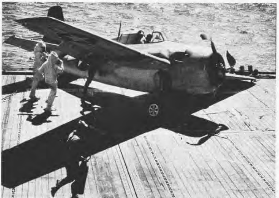
FLOATING IN HIGH, AN FM MISSES ARRESTING GEAR CABLES AND CRASHES ON THE DECK
