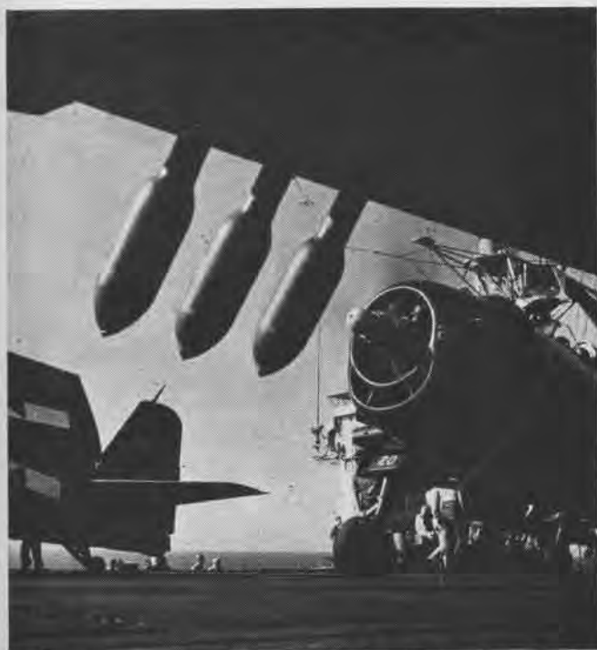
TULAGI'S F6F'S CARRIED ROCKETS WITH 60-LB. BRITISH HEAD
