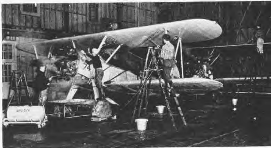
PLANES STARTING THROUGH WASH RACK LINE GET KEROSENE SPRAYED ON ENGINES
