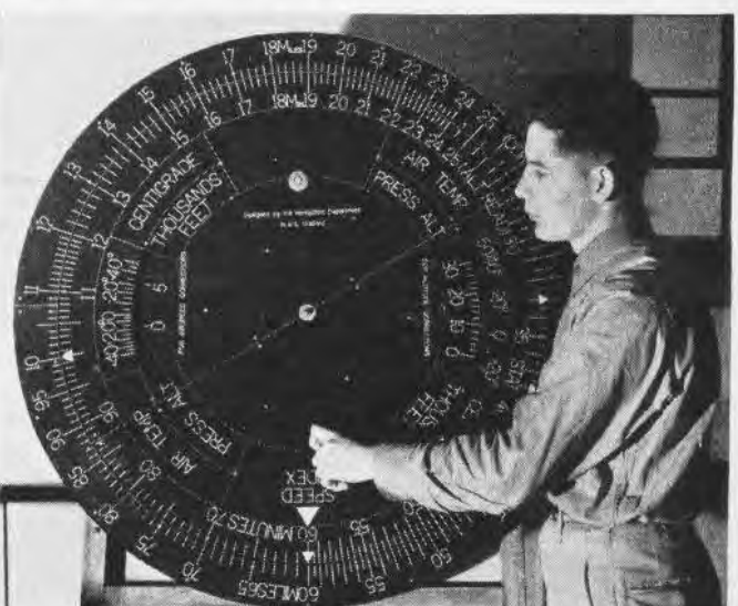
ACCURATE giant model of computer, made from blueprint on plywood base, is valuable aid in navigation class
