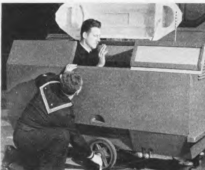
BENDIX CART , synthetic trainer device, can navigate 500 miles inside room, as wheels are geared to distance scale
