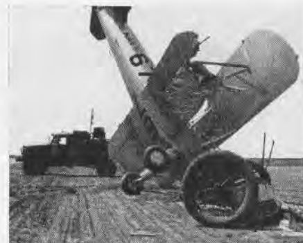
UNORTHODOX LANDING. —This is what happened when a primary student failed to lock out of both sides of his cockpit when he was coming in for landing. Your ball, instructors!
