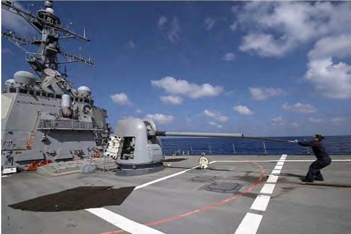
160913-N-ZE250-073 MEDITERRANEAN SEA (Sept. 13, 2016) Gunner's Mate 2nd Class Meghan Smith cleans the barrel of a MK 45 5-inch light weight gun during post fire maintenance aboard USS Carney (DDG 64) while on patrol in the Mediterranean Sea. Carney, an Arleigh Burke-class guided-missile destroyer, forward-deployed to Rota, Spain, is conducting a routine patrol in the U.S. 6th fleet area of operations in support of U.S. national security interests in Europe. (U.S. Navy photo by Mass Communication Specialist 3rd Class Weston Jones/Released)
