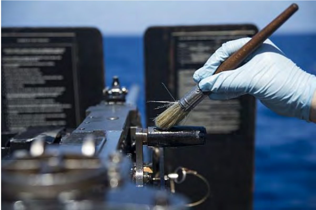
160926-N-ZE250-061 MEDITERRANEAN SEA (Sept. 26, 2016) Fire Controlman 2nd Class Alexander Walsh applies lubricant to an M2 machine gun aboard USS Carney (DDG 64) while on patrol in the Mediterranean Sea. Carney, an Arleigh Burke-class guided-missile destroyer, forward-deployed to Rota, Spain, is conducting a routine patrol in the U.S. 6th fleet area of operations in support of U.S. national security interests in Europe. (U.S. Navy photo by Mass Communication Specialist 3rd Class Weston Jones/Released)
