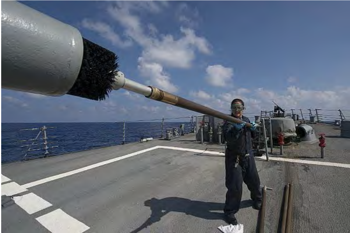
160913-N-ZE250-077 MEDITERRANEAN SEA (Sept. 13, 2016) Gunner's Mate 2nd Class Meghan Smith cleans the barrel of a MK 45 5-inch light weight gun during post fire maintenance aboard USS Carney (DDG 64) while on patrol in the Mediterranean Sea. Carney, an Arleigh Burke-class guided-missile destroyer, forward-deployed to Rota, Spain, is conducting a routine patrol in the U.S. 6th fleet area of operations in support of U.S. national security interests in Europe. (U.S. Navy photo by Mass Communication Specialist 3rd Class Weston Jones/Released)
