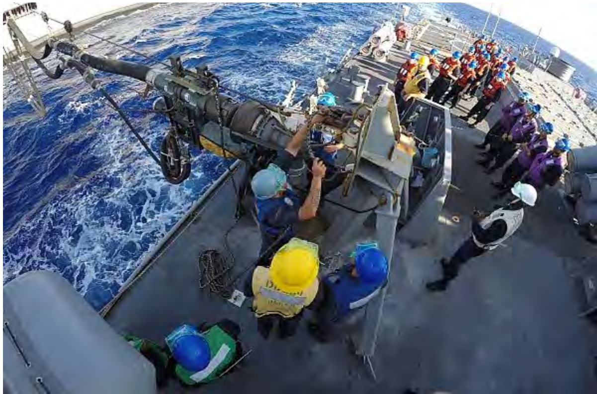
160902-N-ZE250-331 MEDITERRANEAN SEA (Sept. 02, 2016) Boatswain's Mate 3rd Class Daniel Jones inspects the fuel receiving station aboard USS Carney (DDG 64) during a replenishment-at-sea with the Military Sealift Command fleet replenishment oiler USNS Big Horn (T-AO 198) in the Mediterranean Sea. Carney, an Arleigh Burke-class guided-missile destroyer, forward-deployed to Rota, Spain, is conducting a routine patrol in the U.S. 6th fleet area of operations in support of U.S. national security interests in Europe. (U.S. Navy photo by Mass Communication Specialist 3rd Class Weston Jones/Released)
