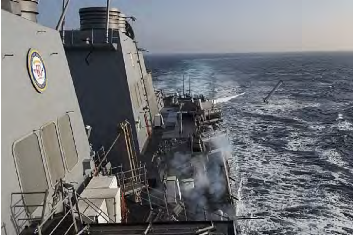
161007-N-ZE250-071 MEDITERRANEAN SEA (Oct. 7, 2016) USS Carney (DDG 64) deploys MK-214 seduction chaff rounds during an air defense exercise in the Mediterranean Sea. Carney, an Arleigh Burke-class guided-missile destroyer, forward-deployed to Rota, Spain, is conducting a routine patrol in the U.S. 6th fleet area of operations in support of U.S. national security interests in Europe. (U.S. Navy photo by Petty Officer 3rd Class Weston Jones/Released)
