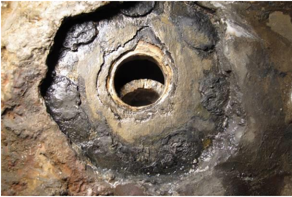
Figure 19. Fractured forward ballast fill line at thru-hull connection, looking inboard.
