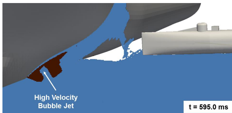
Figure 17. Close up view illustrating the bubble jetting effect. The bubble jet is a high velocity water column that imparts a severe local loading on the hull of USS Housatonic .
