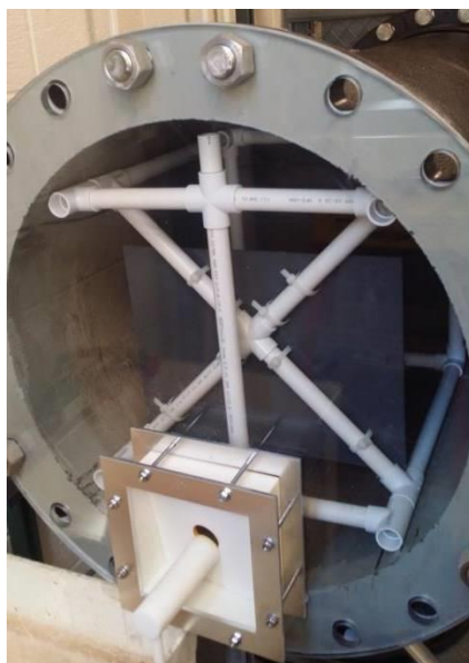
Figure 21. Fracture ballast fill line replica mounted in variable-pressure water chamber
