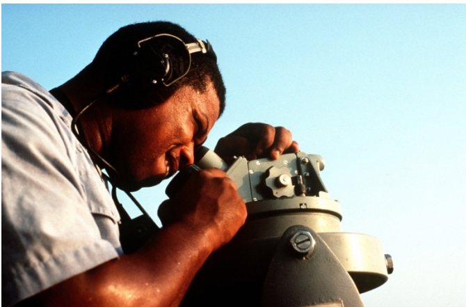
A crewman aboard a minesweeper takes a bearing with a telescopic alidade. Four U.S. Navy minesweepers were deployed to the gulf in support of Operation Desert Shield. (Records of the Office of the Secretary of Defense, 1921-2008)
