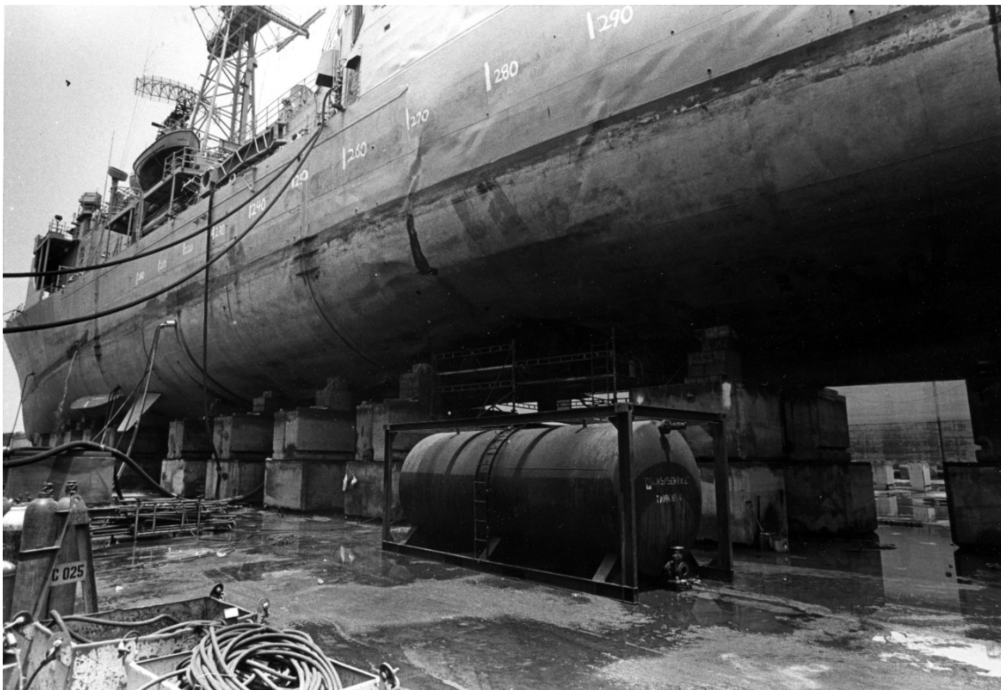
A view of damage to the hull of USS (FFG-58) while in dry dock in Bahrain. The damage was sustained when the ship struck a mine while on patrol in the Persian Gulf on 14 April 1988 (DN-SN-93-01455).
