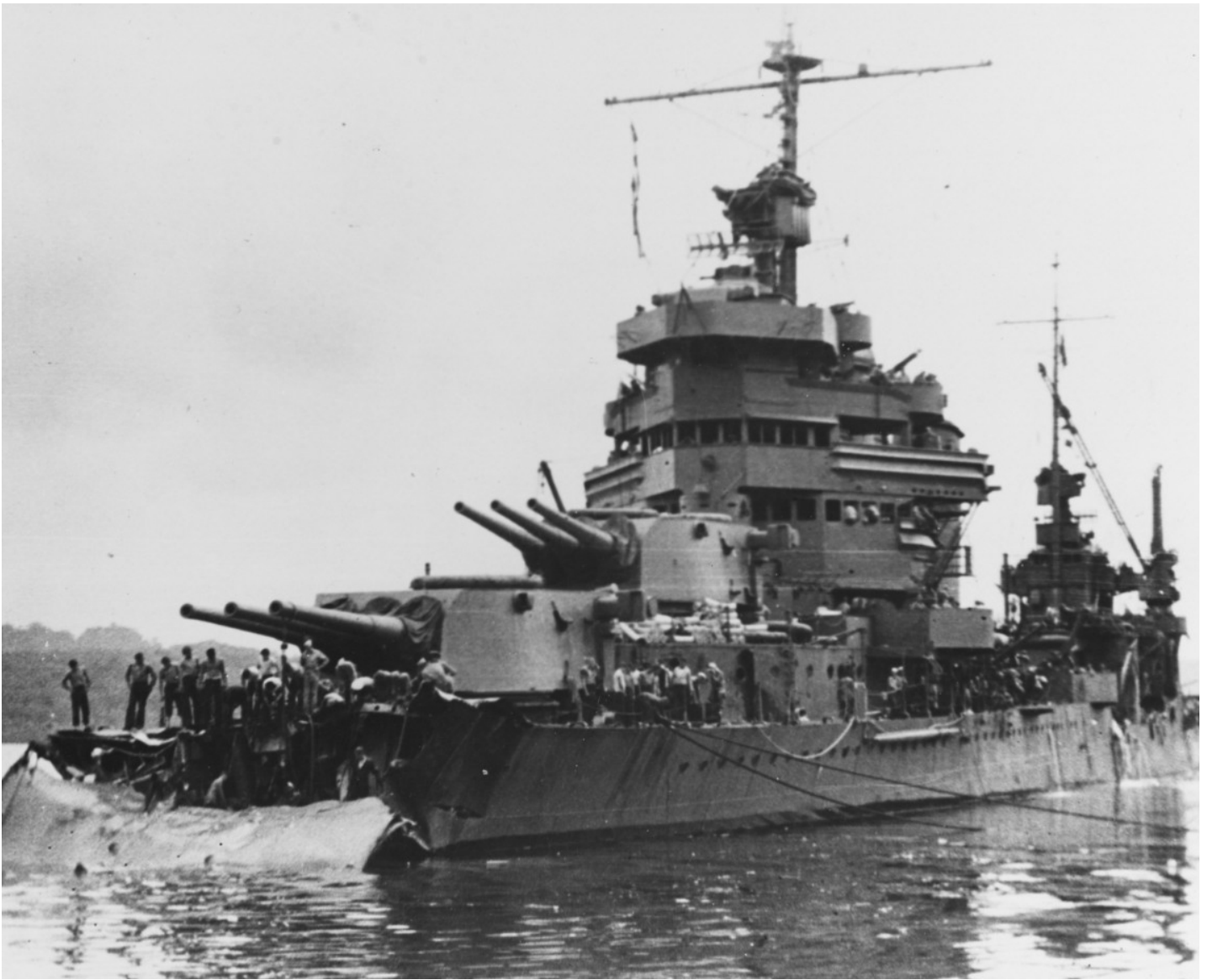
USS Minneapolis (CA-36) at Tulagi with torpedo damage received in the Battle of Tassafaronga. Photograph was taken on 1 December 1942, as work began to cut away the wreckage of her bow (80-G-211215).
