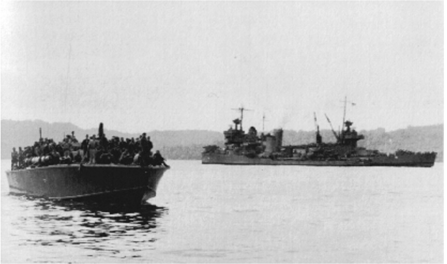
U.S. Navy photo taken after the Battle of Tassafaronga off Guadalcanal shows a U.S. PT boat bringing survivors of the heavy cruiser USS Northampton (CA-26) into Tulagi harbor. In the background is the heavy cruiser New Orleans (CA-32) with her bow blown off, including her number 1 main battery turret. New Orleans survived despite losing almost a quarter of her length.
