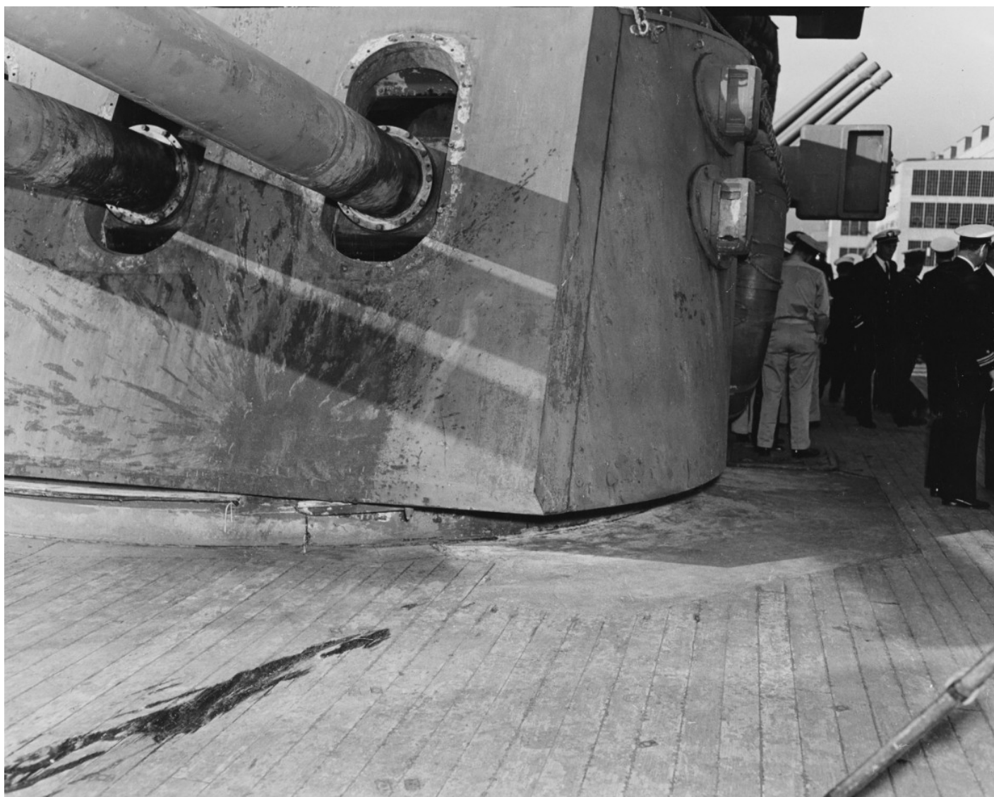
Number 3 6-inch/47-caliber triple gun turret of USS Boise (CL-47), showing the effects of a Japanese shell that struck the turret's 6.5-inch class-A armor face plate during the Battle of Cape Esperance, 12 October 1942. Photographed at the Philadelphia Navy Yard in November 1942, as the ship was receiving repairs. The shell, of unknown caliber, exploded on impact. It did relatively little damage to the armor, but its fragments riddled nearby structure and gouged the turret's guns. The explosion also destroyed the leather gun bucklers (80-G-300232).
