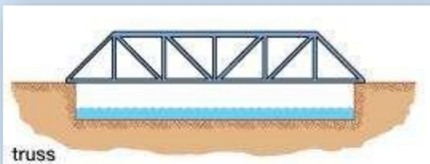
A truss bridge is made up of connecting units in the shape of triangles.
