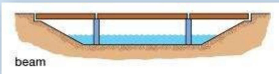
A beam bridge is supported on two ends and can have support columns.
