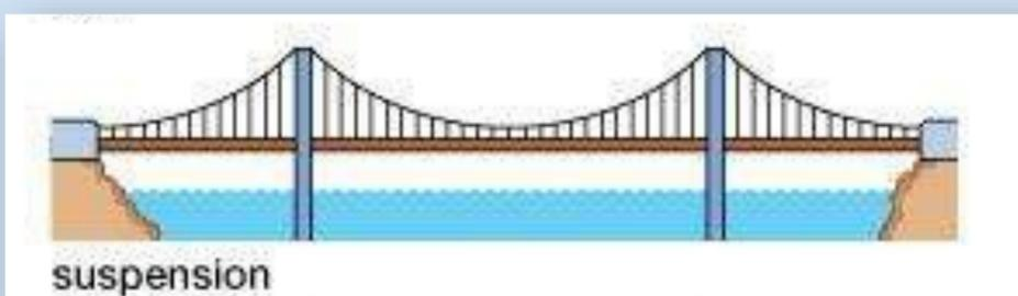
A suspension bridge carries loads through cables.
