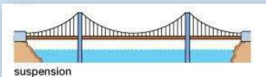
A suspension bridge carries loads through cables.
