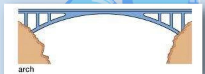
An arch bridge works by transferring loads to each end of the bridge.
