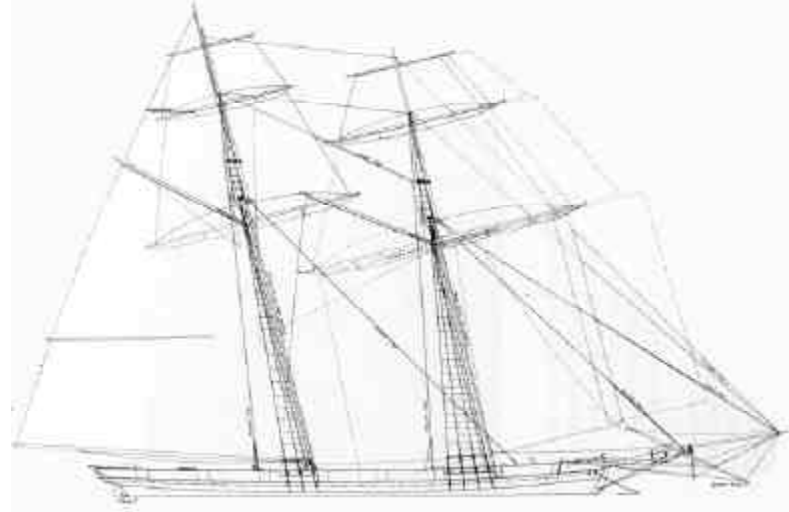
Shown here is a sail plan drawing (i.e. the ship would not carry all these sails) of a Chesapeake Bay-style schooner first developed in Mathews County, Virginia. This later became known as the “Baltimore Clipper” schooner. The vessels’ sharp lines and narrow waist gave it the advantage of speed over heavier British warships. Nine schooner-rigged privateers operated out of Hampton Roads during the War of 1812. (Howard Chapelle drawing of an 1813 privateer)
