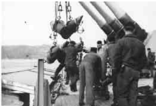
Sixteen-inch shells are loaded on to Wisky while in Sasebo, Japan. The battleship would often race to Sasebo, load up 300 to 400 of the one ton shells and then race back to the bomblines; all this in a little over than 12 hours. (Photo from Wisconsin veterans' collections)
