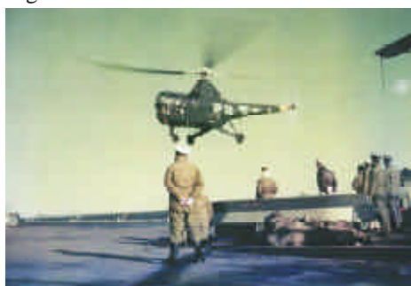
One of the great advances of the Korean War was the use of the helicopter. Wisconsin 's aviation detachment used the Sikorsky HO3S (shown here on BB-64 in December 1951) for spotting targets on shore and for search and rescue of downed aviators. (Photo from Wisconsin veterans collections )
