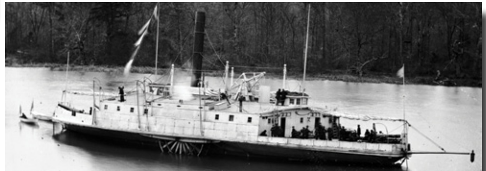
This is USS Commodore Morris photographed on the James River. This image gives an excellent overview of the best and worst qualities of ferryboats as warships. Notice the boiler plates along the side of the ship. After the war, Commodore Morris served once again as a New York City ferryboat until 1931. (Library of Congress image)
