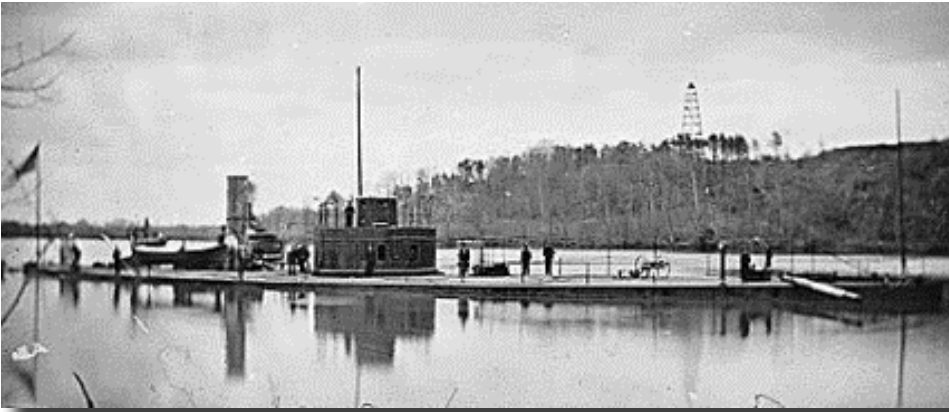
The threat of the Confederacy's James River Squadron's ironclads, whether they were in working condition or not, forced the U.S. Navy to keep at least one monitor-type ironclad on duty in the James River at all times. Shown here is the 1,300-ton USS Lehigh which was equipped with the new XV-inch Dahlgren smoothbore. (Library of Congress image)
