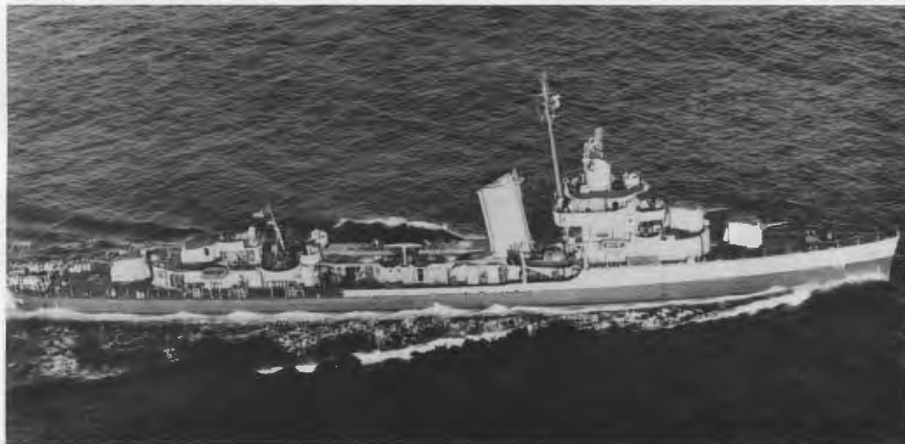
The Norfolk-built and based destroyer USS Wainwright (DD-419). The 1570-ton destroyer was a well armed vessel equipped with four five-inch dual purpose guns, eight torpedo tubes, eight machineguns, and depth charge racks. She began her combat career in 1942 on the most dangerous convoy route of the war. (U.S. Navy photo)
