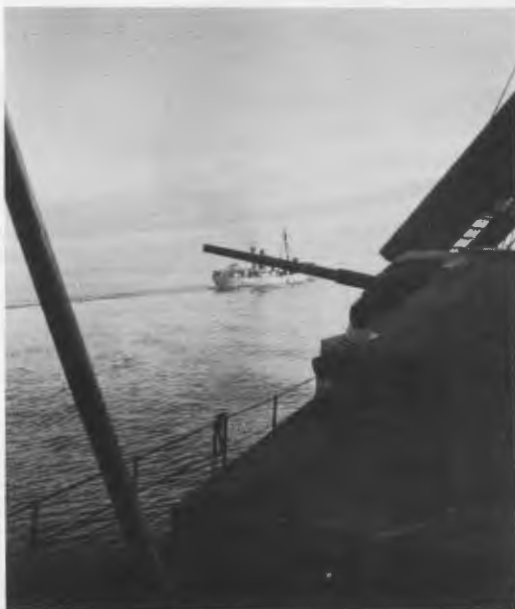
Lacking adequate anti-aircraft guns, enterprising U.S. Naval Armed Guard sailors rolled out M-3 Lee-Grant tanks that were meant for the Russians onto the decks of the merchant ships during the PQ-17 operation. (U.S. Navy photo)
