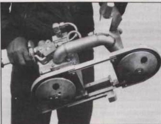
A new seawater hydraulic band saw for cutting armored cable and pipe up to four inches in diameter. The one-of-a-kind tool is an improved version of the Laboratory's oil hydraulic saw. It can cut through a 3½-inch diameter double-armored cable in approximately one minute.
