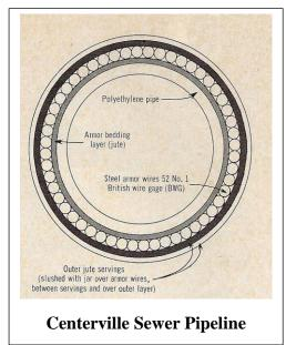
contained 1,000 feet of pipeline which could be deployed from the reel using the same techniques used for laying undersea cables.
