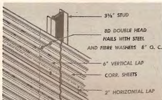
DETAIL SHOWING BULKHEAD CORRUGATED SHEET LAP
