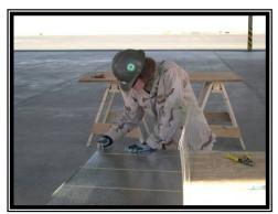
A Seabee fabricates ductwork.
