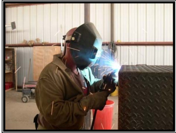
A steel worker builds a junction box.
