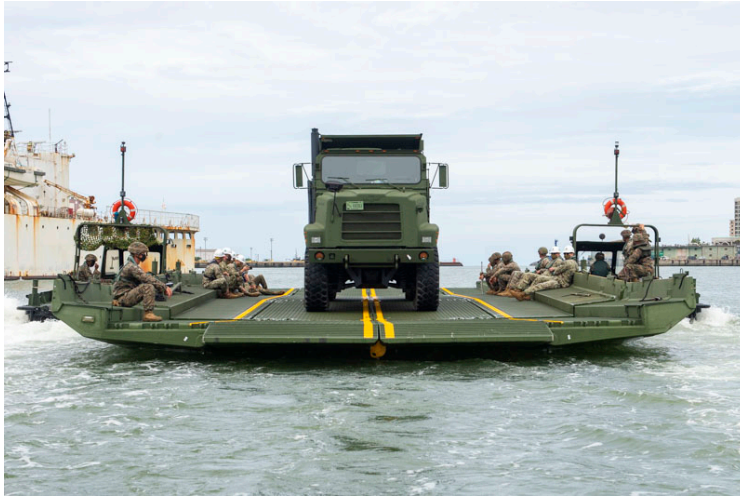
Seabees and Marines assigned to Bridge Company, 9 th ESB, 3 rd MLG demonstrate the employment of an IRB to transport CESE.
