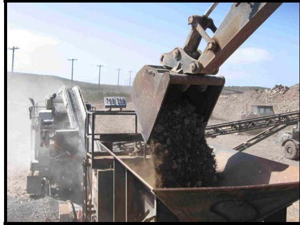
Crushing 4" Minus Rock to ¾" Minus
