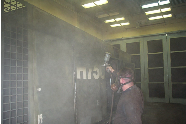
Painting 750 CFM Air Compressor
