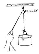
Pulley – pulleys use a similar wheel and axle to reduce the effort it takes to lift an object. Using more than one pulley reduces the amount of effort required to lift an object. If you ever get a chance to see a crane in action, they use a system of pulleys to lift heavy objects.
