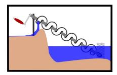
Screw – a screw uses the same principles as the incline plane, using a circular function, as objects move up and around the plane. Screws can be used to pull a large amount of materials from one location to another, particularly if your screw has a tube like the one pictured here. There are screws in many
