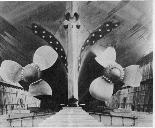
The 8,600 ton Glacier in Wellington, N.Z., drydock. Each propeller is 17½ feet in diameter, blades were broken in McMurdo Sound in December.
