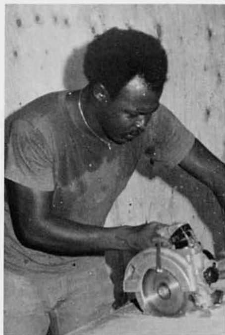
ABOVE: BU3 Smiley cuts forms in the carpenter shop.
