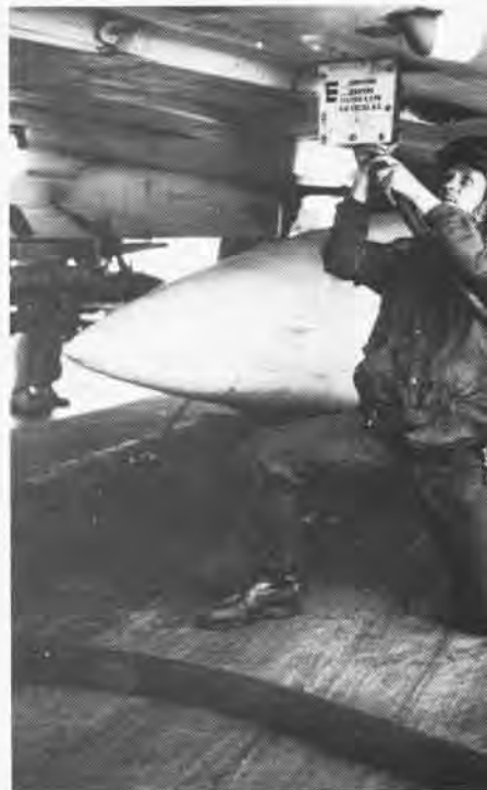
Hooking up the power connection, the plane captain prepares his aircraft for launch, above. The pilot and plane captain use hand signals as they check the aircraft's movable parts, below. Before and after each launch, the squadron plane captains can be seen dragging chains at their sides, below left.
