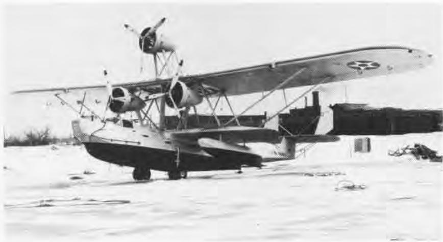
The XP2Y took off faster with only two engines; the third created more drag.
