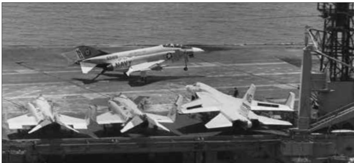
An F-4J lands on Constellation (CVA 64), 29 July 1974. The F-4 was originally designed as a fleet defense fighter but was utilized extensively in Vietnam as a bomber as well. It could achieve speeds in excess of Mach 2 and carry up to 18,650 pounds of ordnance, including air-to-air missiles and laser-guided bombs. Its powerful pulse-doppler radar was a supreme technological breakthrough at the time. It could identify targets well beyond visual range and direct radar-guided Sparrow missiles at MiGs up to 12 miles away.
