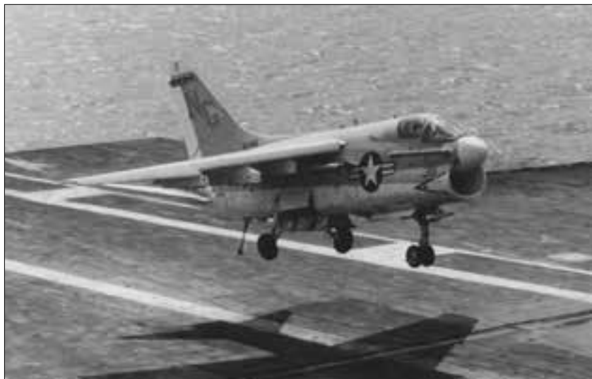
An A-7E Corsair II landing on the flight deck of Ranger (CVA 61), January 1968. The A-7 proved a highly successful attack aircraft during the final years of the Vietnam War. It could fly up to Mach .94 and featured a sophisticated bombing computer and all-weather navigation system.
