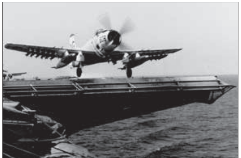
An armed A-1 Skyraider launches from aircraft carrier Ranger (CVA 61). The great fuel and armament capabilities of the propeller-driven planes made them valuable assets in search and rescue missions.
