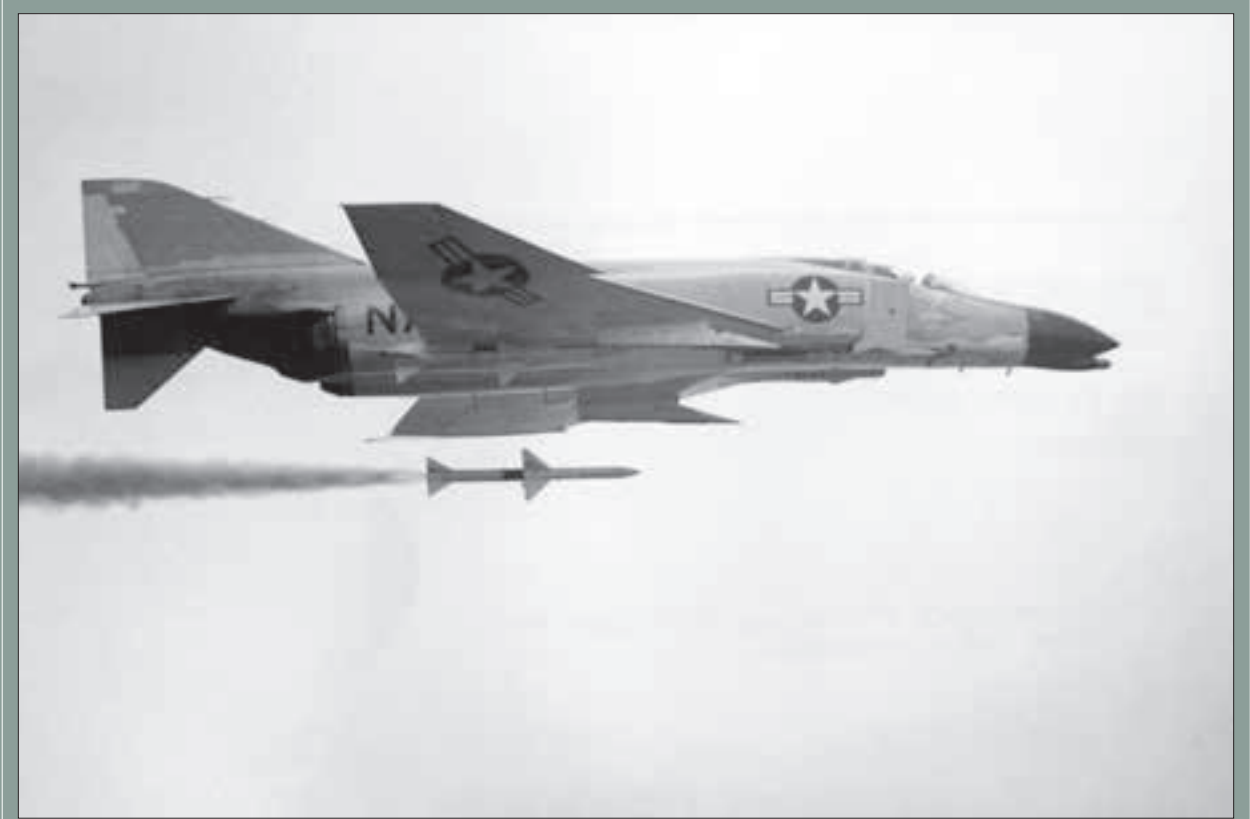
An F-4 Phantom II, based at Point Mugu Naval Air Station, California, fires a Sparrow III air-to-air missile in preparation for combat operations in Southeast Asia.
