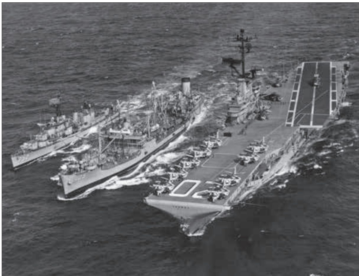
Aircraft carrier Bennington (CVS 20) and destroyer Alfred A. Cunningham (DD 752) refuel from fleet oiler Mispillion (AO 105) while underway.
