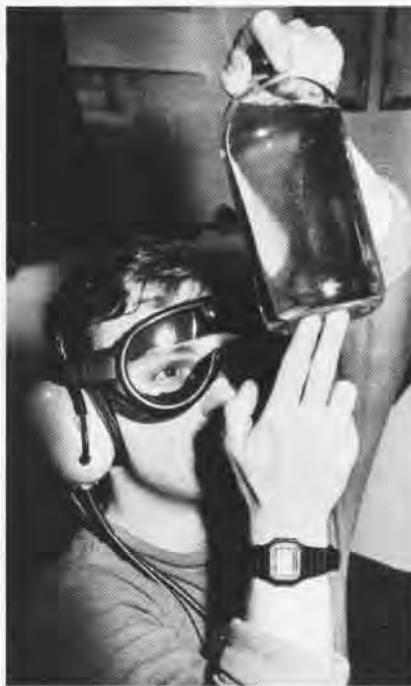
ABF3 Mark Mooney checks an aircraft fuel sample for water and sediment aboard Independence (CV 62).
