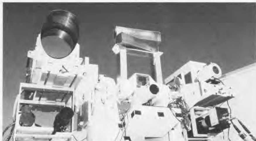
Sensors on a Kineto tracking mount follow an incoming target.
