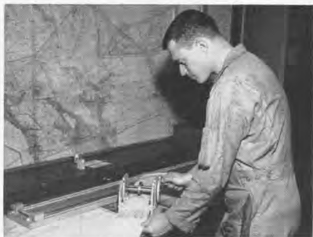
USING A "Rube Goldberg" device, Ltjg. Walt Wattenburger punches holes along the strip chart edges to match the pegs on the roller.
