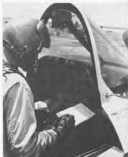
FOUR KNEE-PAD pages are filled with readings, "sat" or "unsat," and remarks for test flight.
