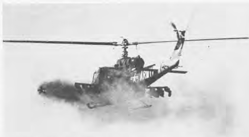
ARMY HU-1A Iroquois helicopter demonstrates ability to let loose a lethal barrage of six SS-11 guided wire missiles during trials. Now in service with field units, HU-1A handles suppressive fire missions without sacrificing speed or maneuverability.
