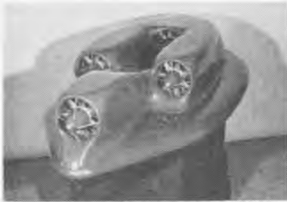
GEM CRUISE configuration of David Taylor Model Basin's Model Aerodynamics lab to determine its pitch, lift and drag characteristics at various engine revolutions and angles of attack. 48 ground effect machine goes through wind tunnel tests in
