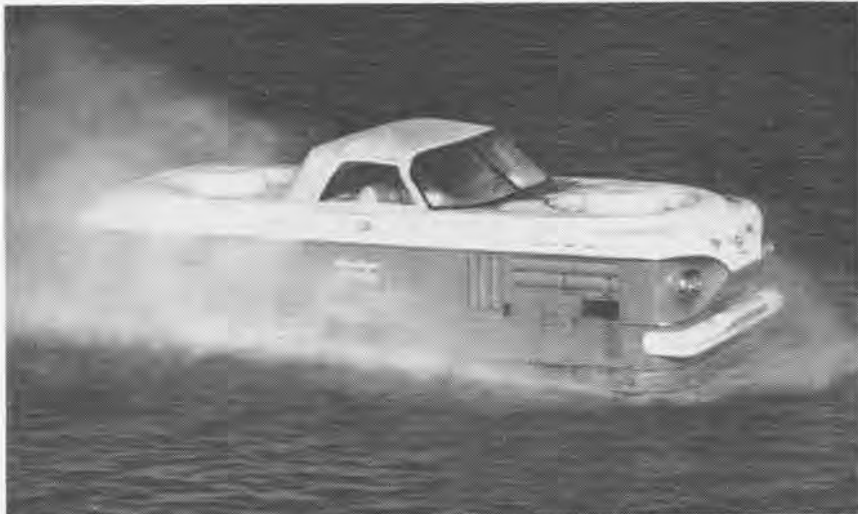
CURTISS-WRIGHT air car has land and water capability. It made 53 mph in this test at Daytona. The Army bought two of these annular jet GEMs for its testing program.
