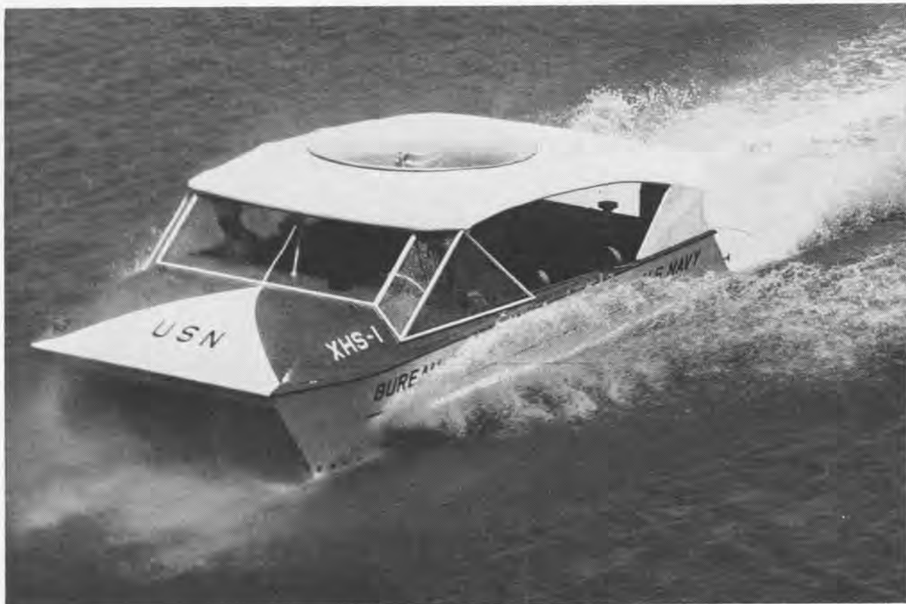
HUGHES XHS-1 Hydrostreak skims over water on cushion of air. Two skegs, one on either side of hull, and a waterwall at each end trap air to form the cushion. The propeller increases speed.
