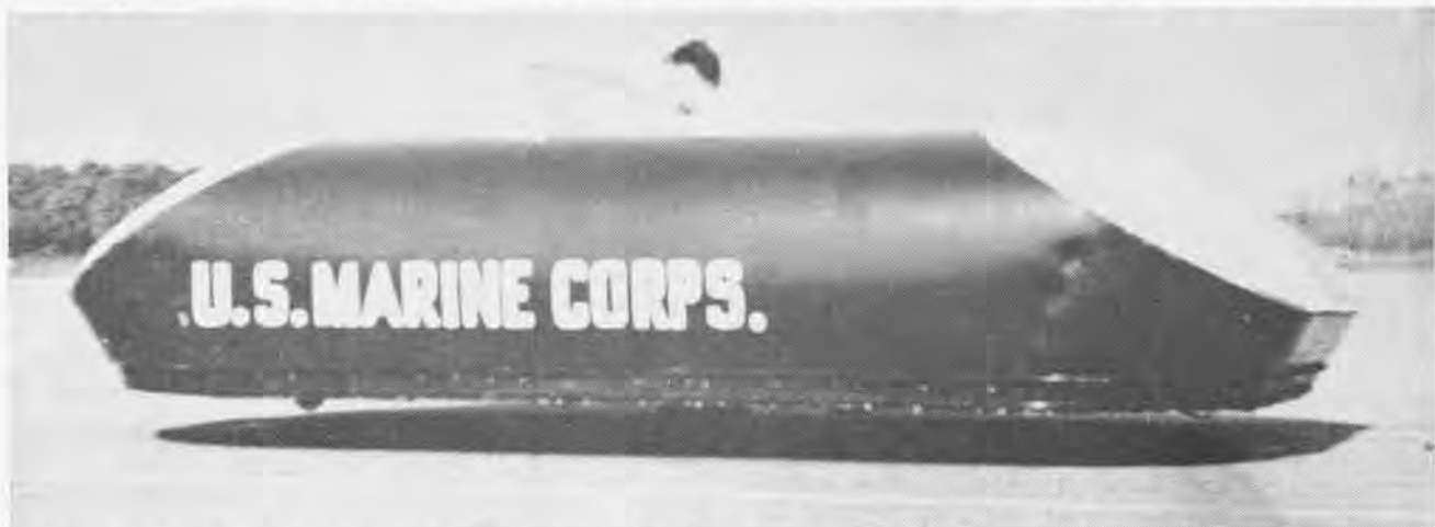
NATIONAL RESEARCH Associates' Pegasus I has been tested by Marines at Quantico. Supporting air cushion is generated by four low pressure fans, two at each end. Can lift gross weight of 1100 pounds to height of 15 inches and can make up to 60 mph.
