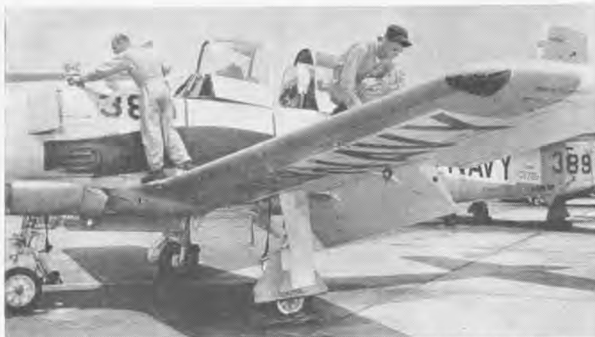
TEST FLIGHT is key inspection in VT-3's quality control program. Here test pilot Walljasper checks the oil while his crewman Little gets fuel in a thorough pre-test flight inspection.
