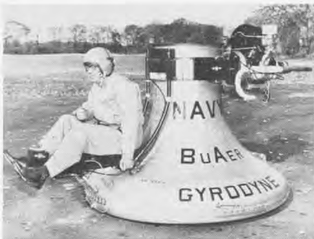
GYRODYNE MODEL 55 GEM , authorized in 1959, employs annular jet principle. A one-man vehicle, it uses a Porsche engine.
