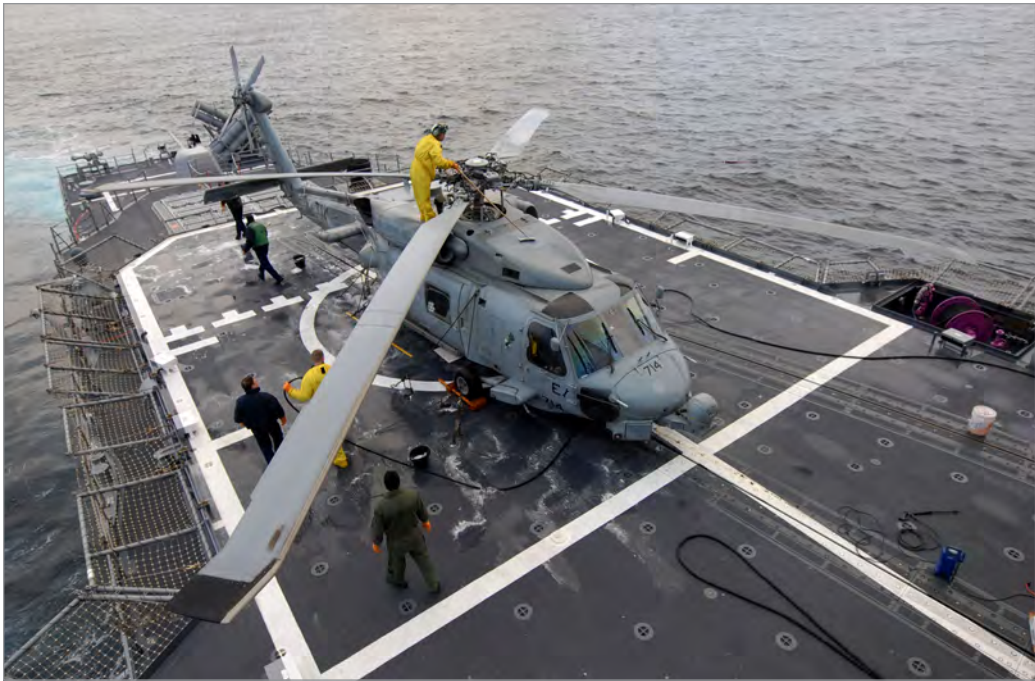
Sailors decontaminate an SH-60B Seahawk helicopter assigned to HSL-51 on the flight deck of the guided missile cruiser Shiloh during Operation Tomodachi. (Seaman Charles Oki, USN; 23 March 2011; DVIDS, 382013)
