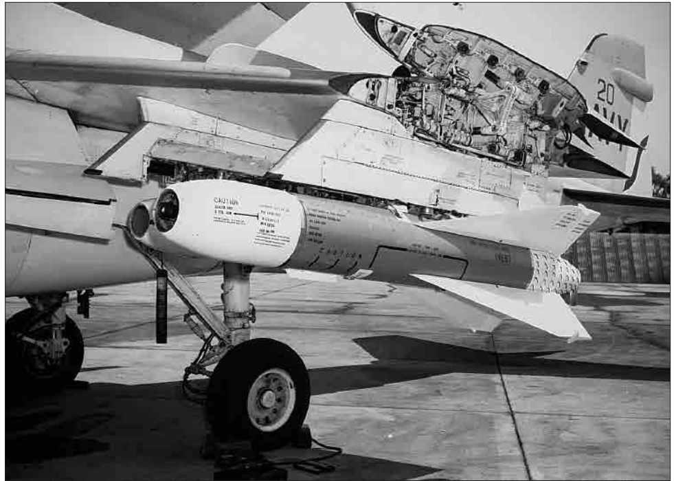
An inert Walleye television-guided air-to-surface glide bomb with string tufts attached to its aft section is mounted on an A-6 Intruder for aerodynamic testing.
