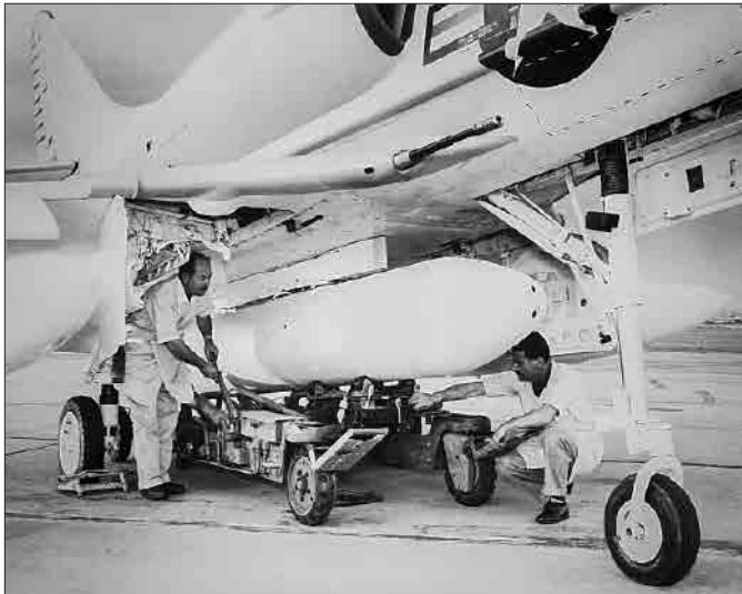
A Mk 11 20mm gun pod is mounted onto an A4D-2 Skyhawk at the 1958 Naval Air Weapons Meet in El Centro, Calif., during the weapon's test phase by the Naval Aviation Ordnance Test Station in Chincoteague, Va.
