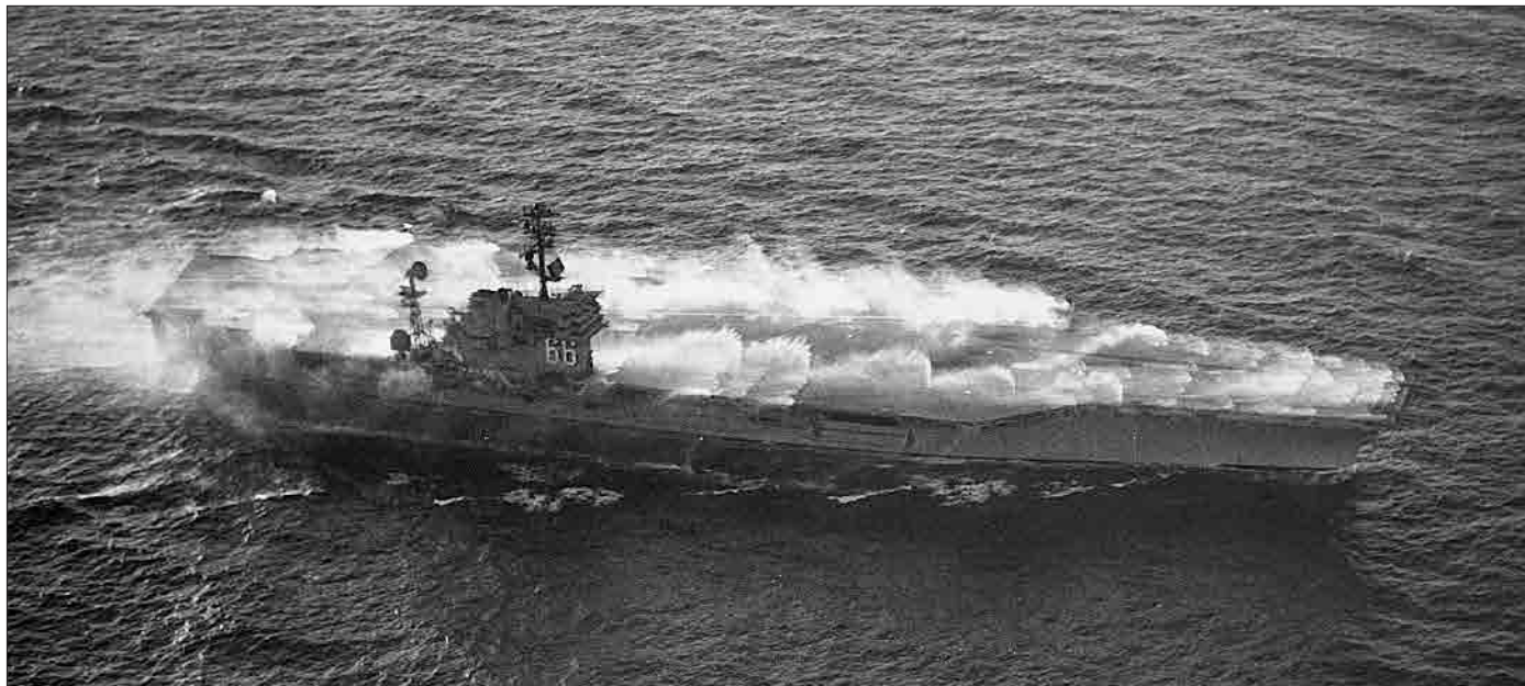
America (CVA 66) tests her water washdown system for firefighting. The flush-deck nozzles can provide up to 27,000 gallons of water per minute.
