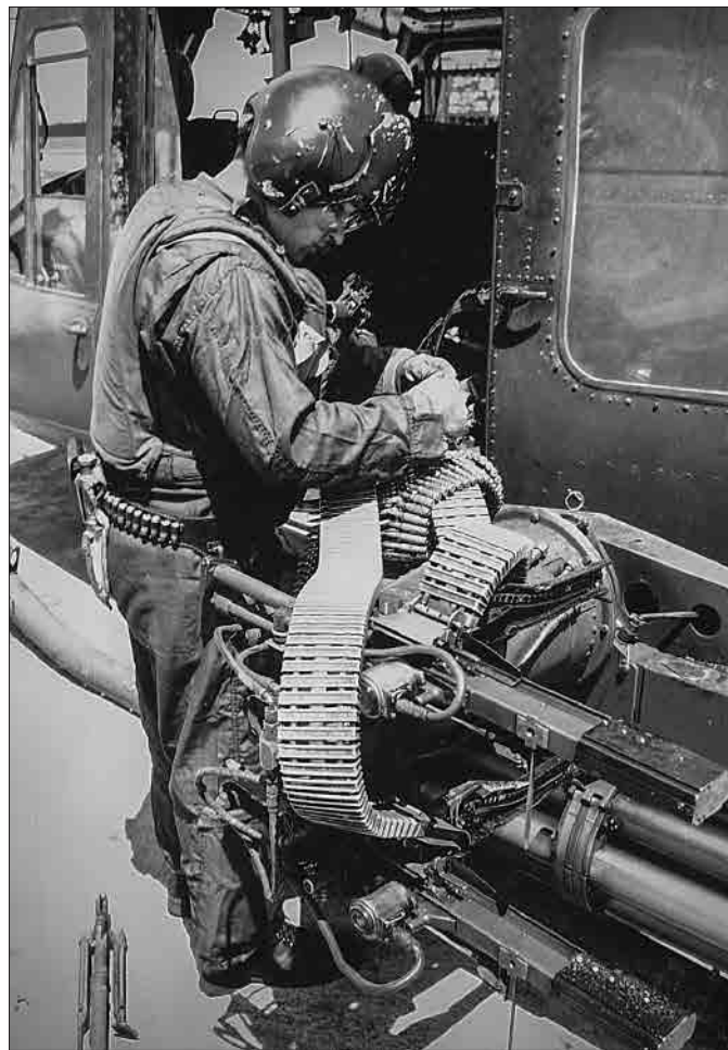
A crewmember reloads an M-60 machine gun on a Marine UH-1E Iroquois.
