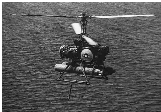
DS-1382, shown modified as the first QH-50D, was one of 373 DSN-3 (later QH-50C) drone antisubmarine helicopters built. It is carrying two Mk 44 torpedoes.
