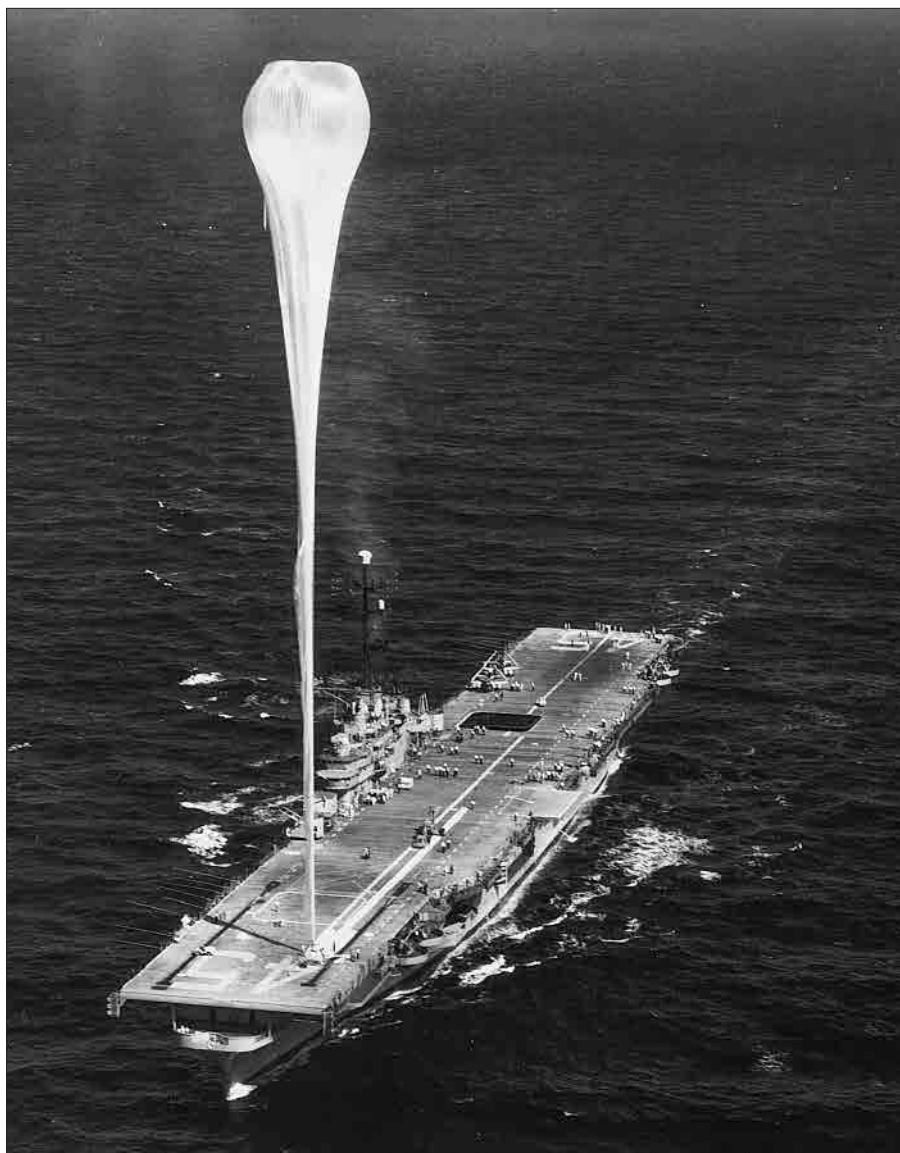
Valley Forge (CVS 45) prepares to launch a Project Skyhook unmanned balloon to record cosmic ray activity, 26 January 1960.
