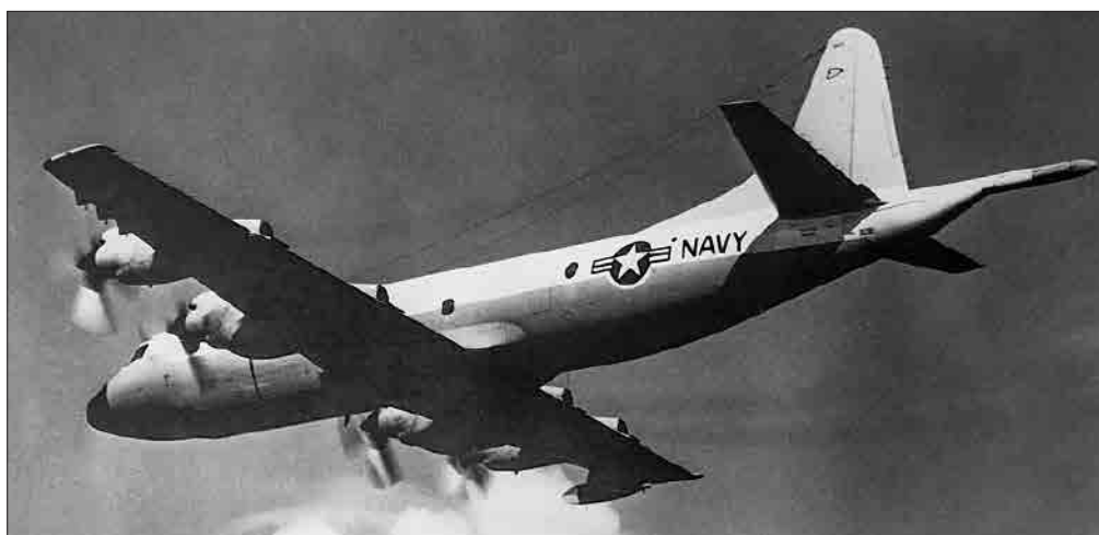
The P-3A Orion antisubmarine patrol plane is a derivative of the Lockheed L-188 Electra passenger airliner.
