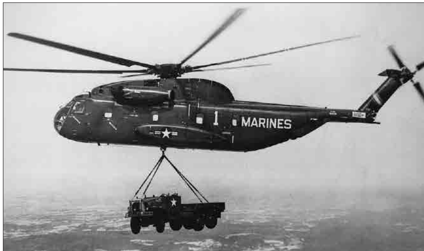
The eighth Marine CH-53A Sea Stallion built, BuNo 151691, displays its heavy-lift capability. The type first entered service in 1966.
