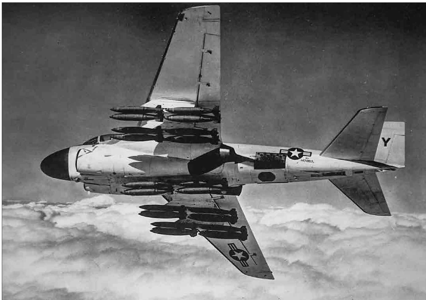
The fourth YA2F-1 Intruder, BuNo 147867, shown here, was the first fitted with the full set of advanced electronic systems which enabled later version A-6s to penetrate enemy defenses and to bomb through the clouds.
