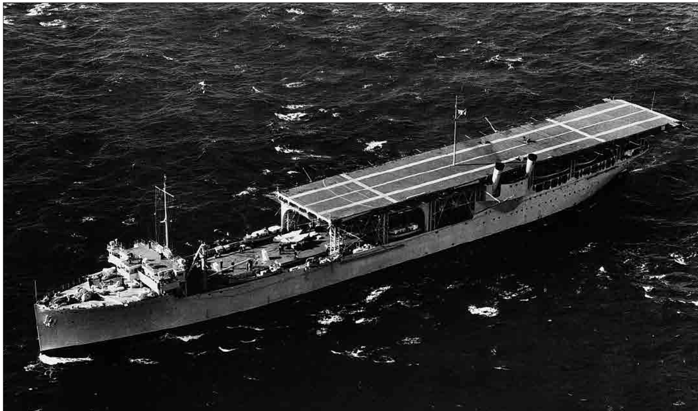
Langley (AV 3) following her conversion to a seaplane carrier, including the removal of the forward flight deck.
