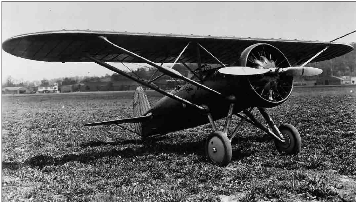
The XF5B-1, the Navy's first monoplane designed for carrier operations.
