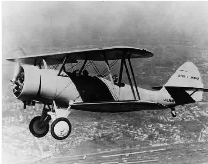
An XN3N-2 "Yellow Peril" trainer built at the Naval Aircraft Factory, Philadelphia, Pa.
