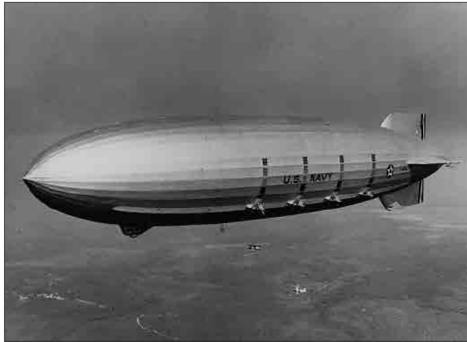
F9C-2 Sparrowhawks return to their mothership, the rigid airship Macon (ZRS 5). Her hangar bay could accommodate five of the little fighters.
