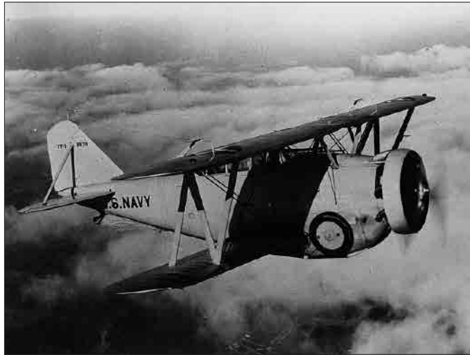
An FF-1 fighter, the first naval aircraft to incorporate retractable landing gear.
