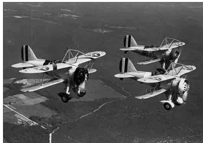
A trio of F9C-2 Sparrowhawks fitted with airship hook-on gear.
