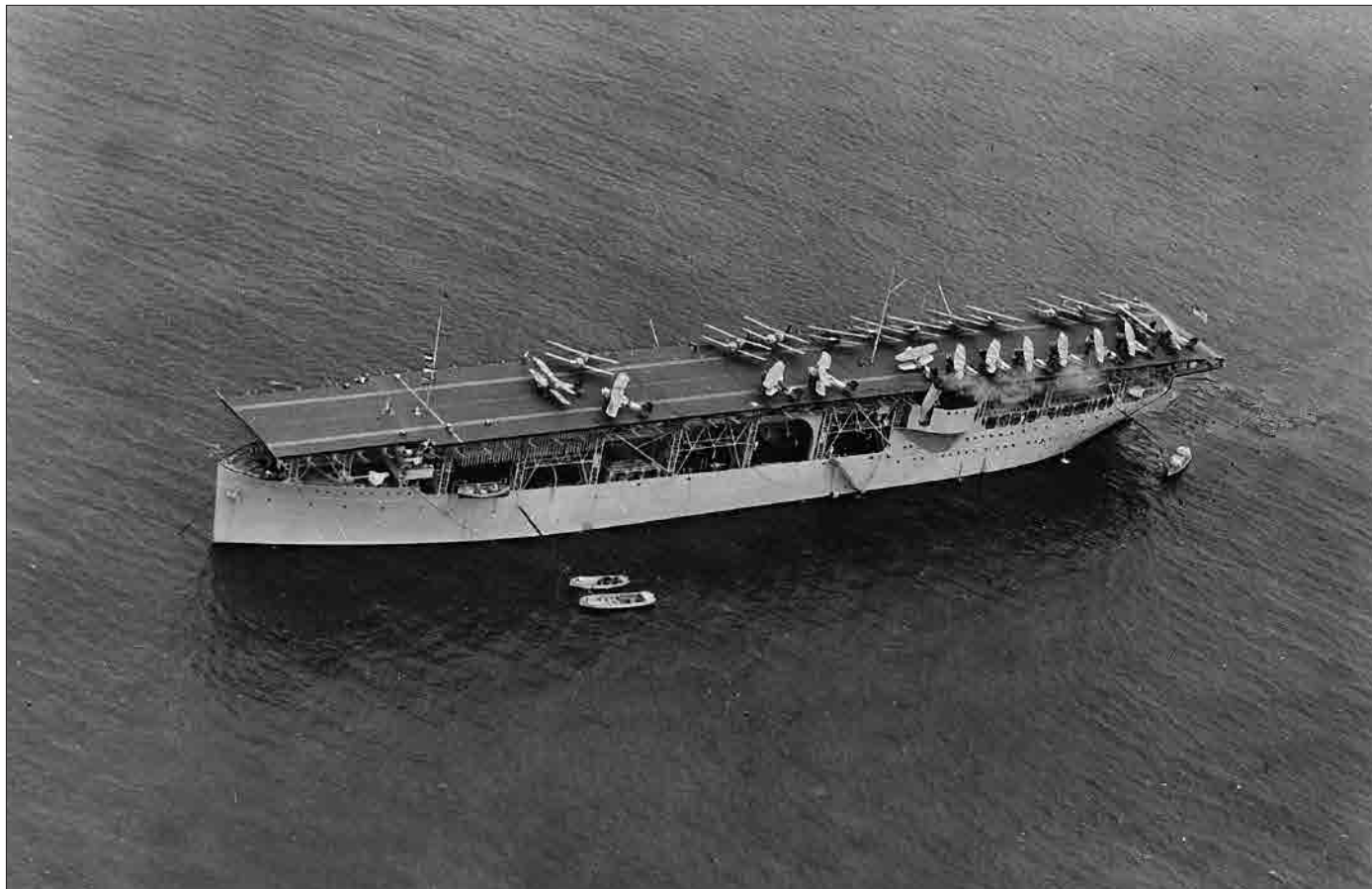
Fighters and torpedo planes pack the deck of the first U.S. aircraft carrier, Langley (CV 1).
