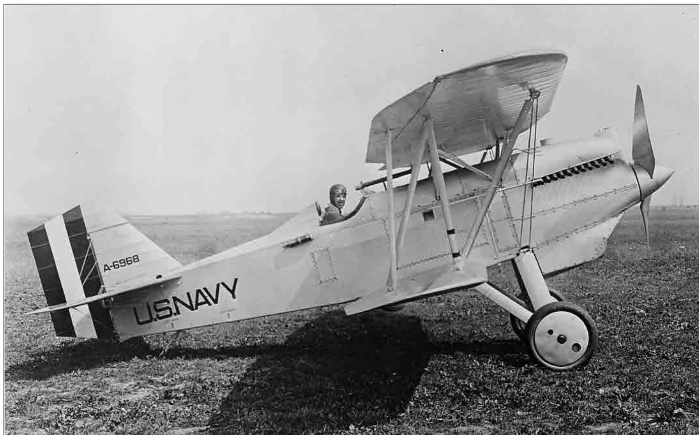
A D-12 engine powers this F6C-1 fighter, which later became the prototype F6C-4.
