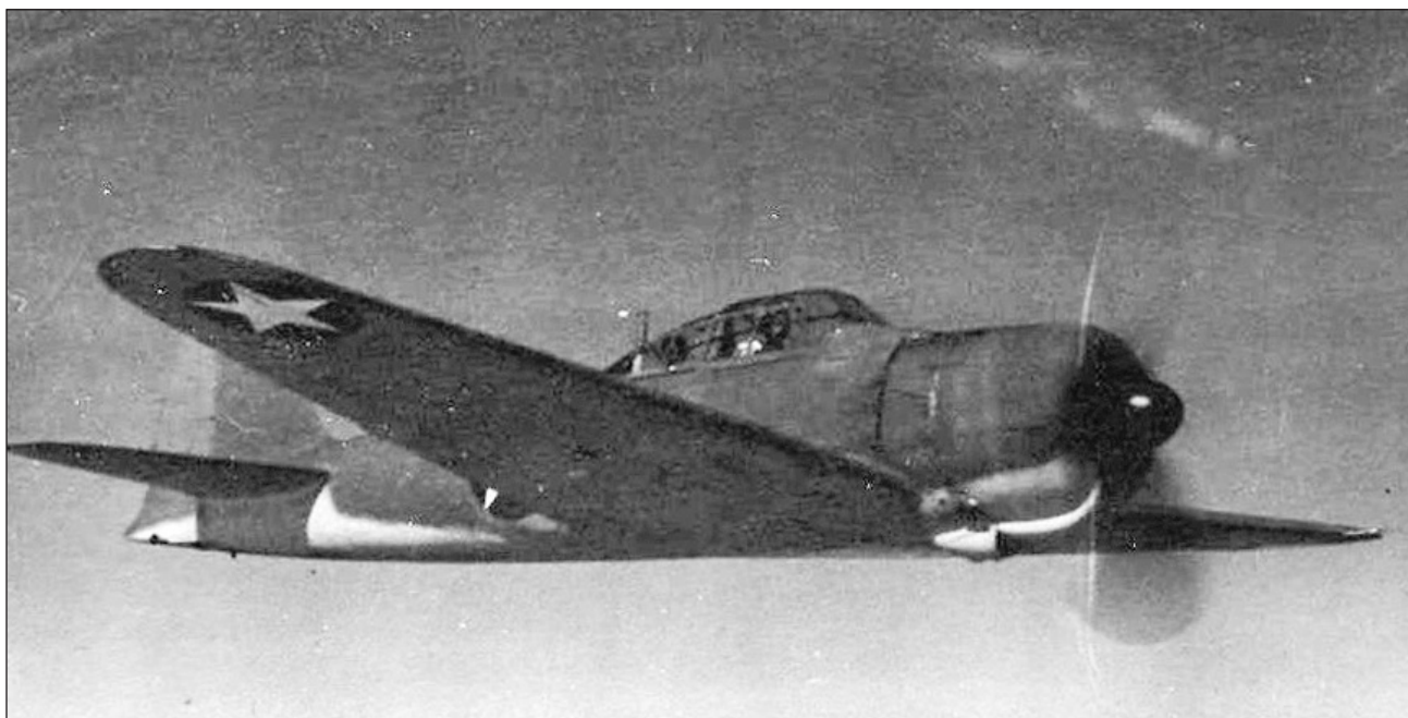
This is the Japanese Mitsubishi "Zero" fighter, which began appearing in Pacific combat zones about the time of the Coral Sea battle. It was a highly maneuverable craft, but limited in fire power and without armor or self-sealing fuel tanks. Out pilots found them worthy opponents. The one pictured here was captured in the Aleutians, which accounts for the United States insignia.
