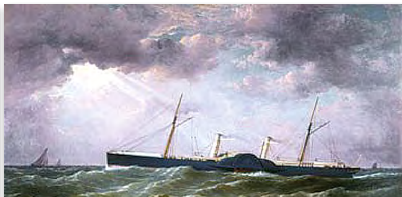
The Civil War produced the requirement for a lighter material for speed-hungry blockade runners. Thus, British shipyards began using steel in large quantities in their new blockade runners (shown here are Armstrong at left and Banshee at right). While blockade runners reached the desired speed, the ships would often enter port with the hulls literally falling apart. (Museum of the Confederacy and NHHC images)
