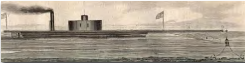
Ericsson's invention to counter Confederate torpedoes was a wooden raft that would set off the torpedo prematurely. It is shown here on USS Weehawken (Harpers Weekly engraving)
