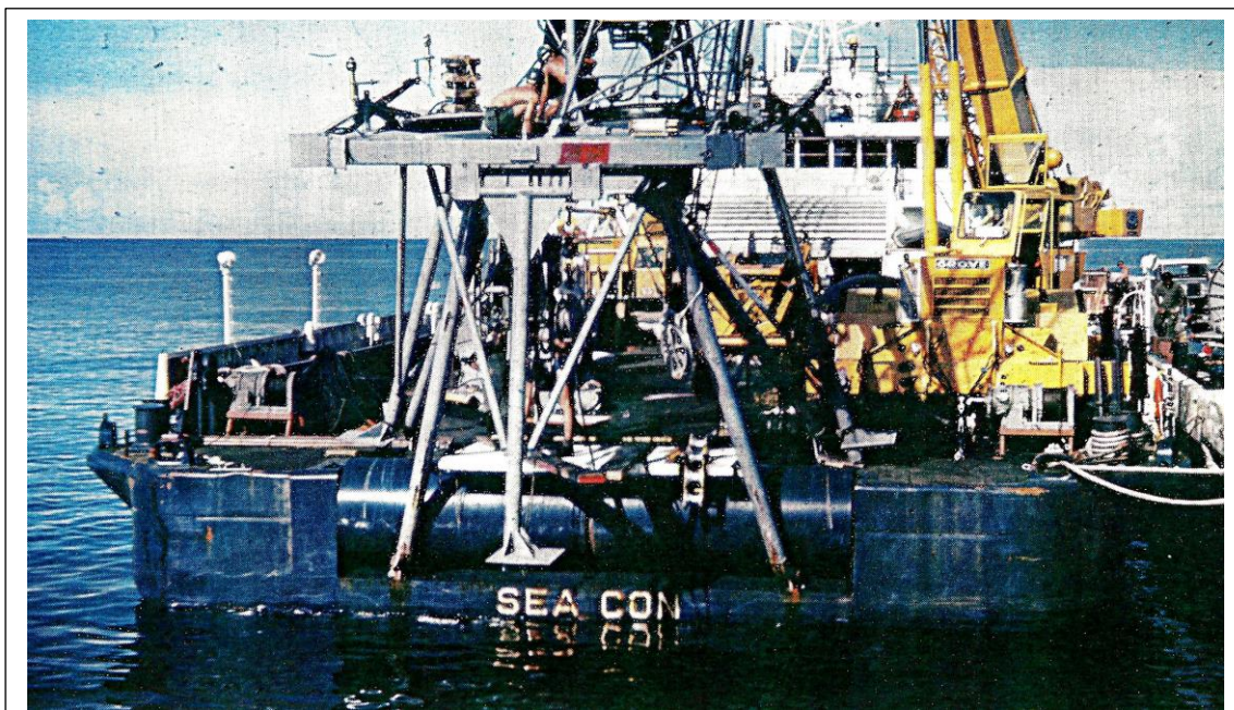
New Hydrophone Array Loaded on SEACON Ready to be Offloaded
